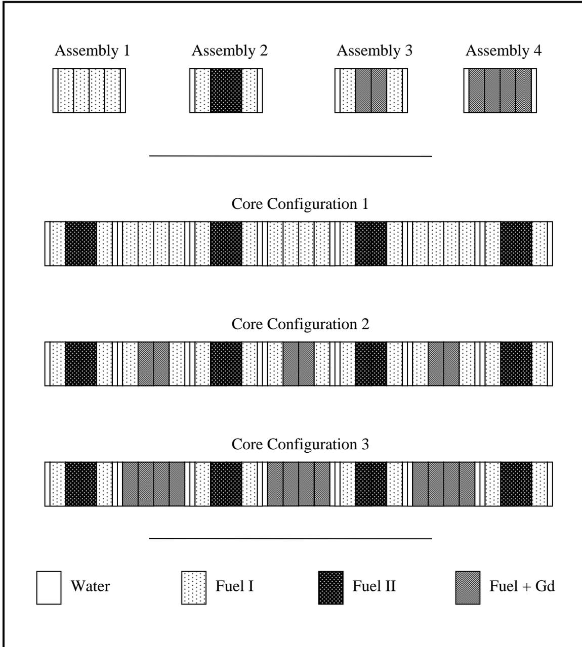
**Figure A.1. Assembly and Core Composition and Geometry**
