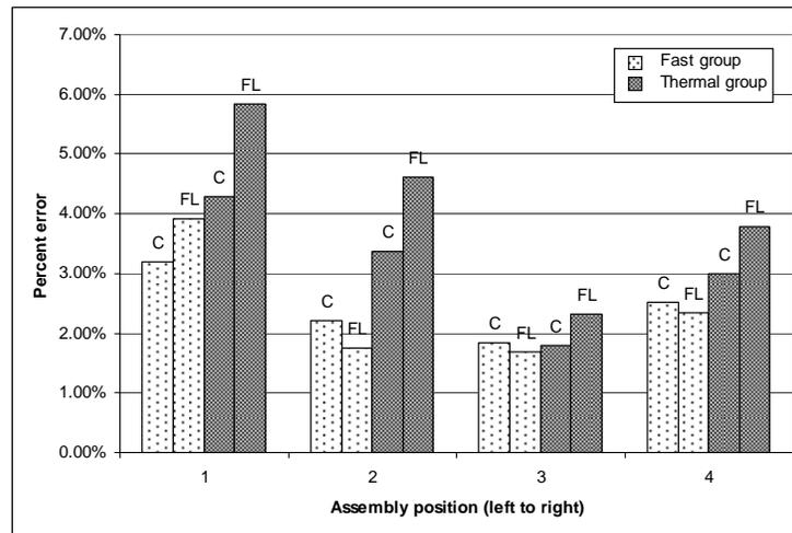
Figure 5. Average Flux Errors in Core 3
