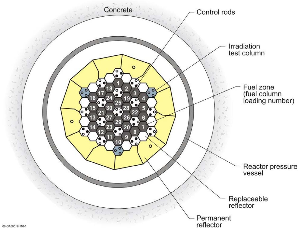
**Figure 2. Horizontal Cross Section of the HTTR.**
