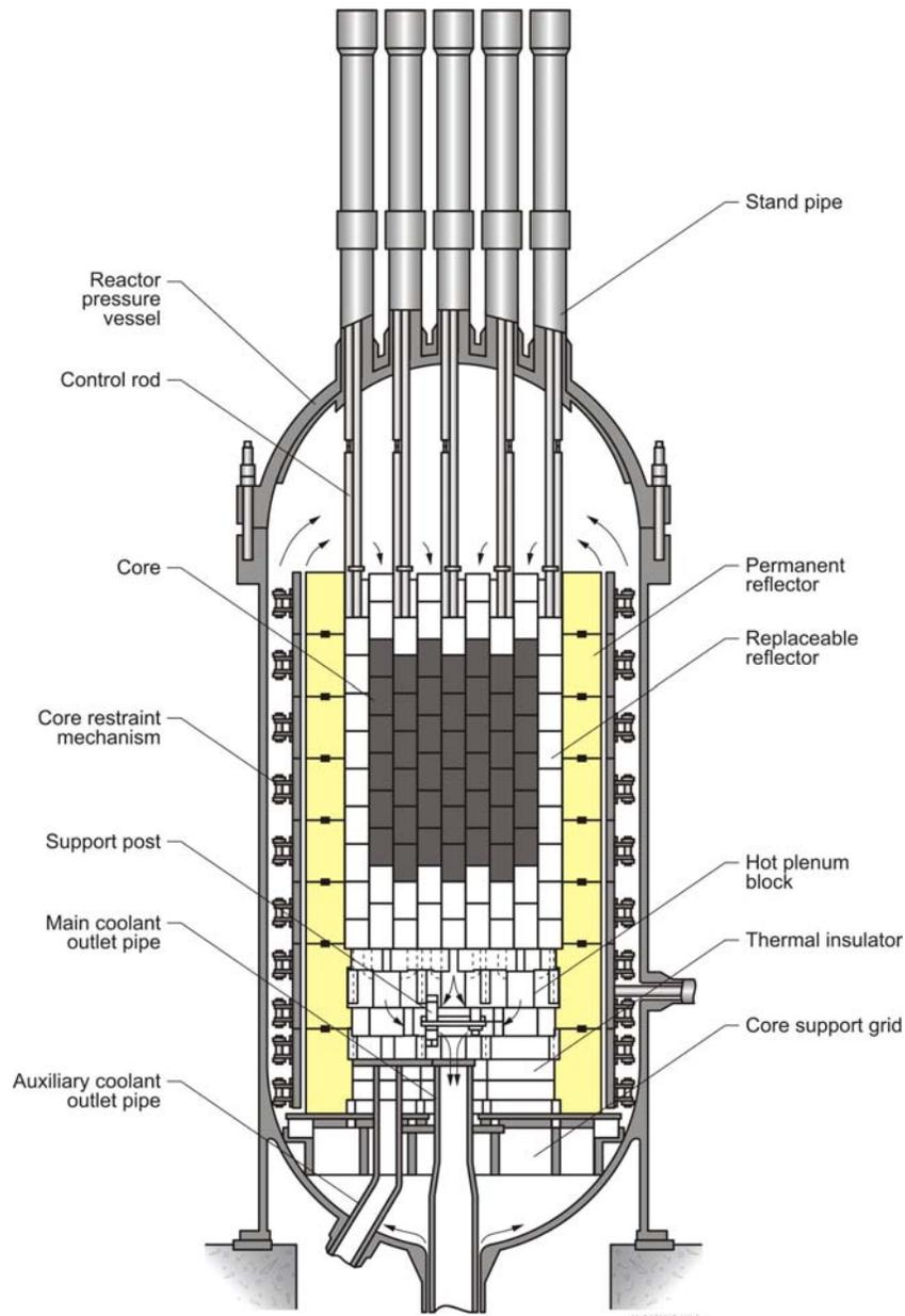
**Figure 1. Vertical Cross Section of the HTTR.**
