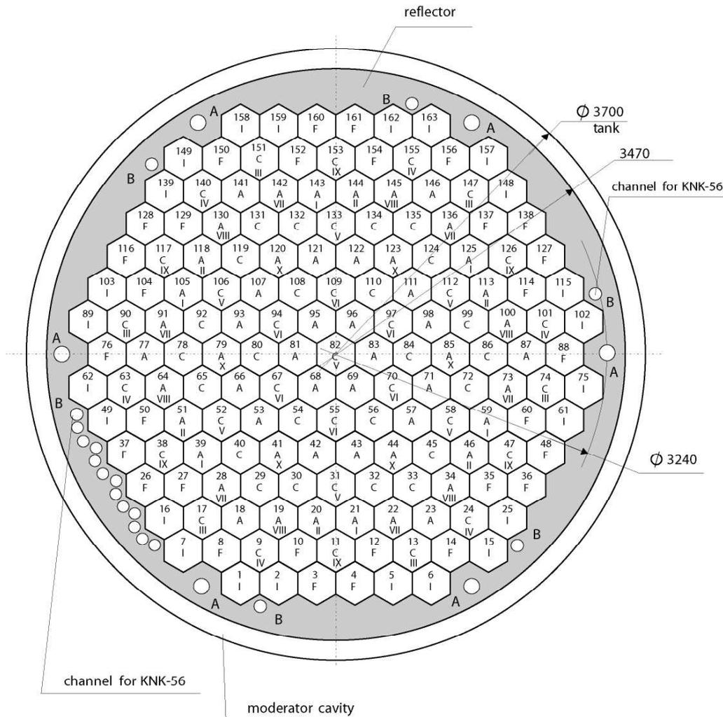
**Figure 1. Radial geometry of V-1000 core (VVER-1000 mock-up). VVER-1000 first cycle loading with U-235 enrichments: A - 1.6 %, C - 3.0 %, F - 4.4%+3.6% (profiled), I - 4.4 %. Control rod group numbers denoted by Roman numerals. KNK: out-core ionization chambers.**
