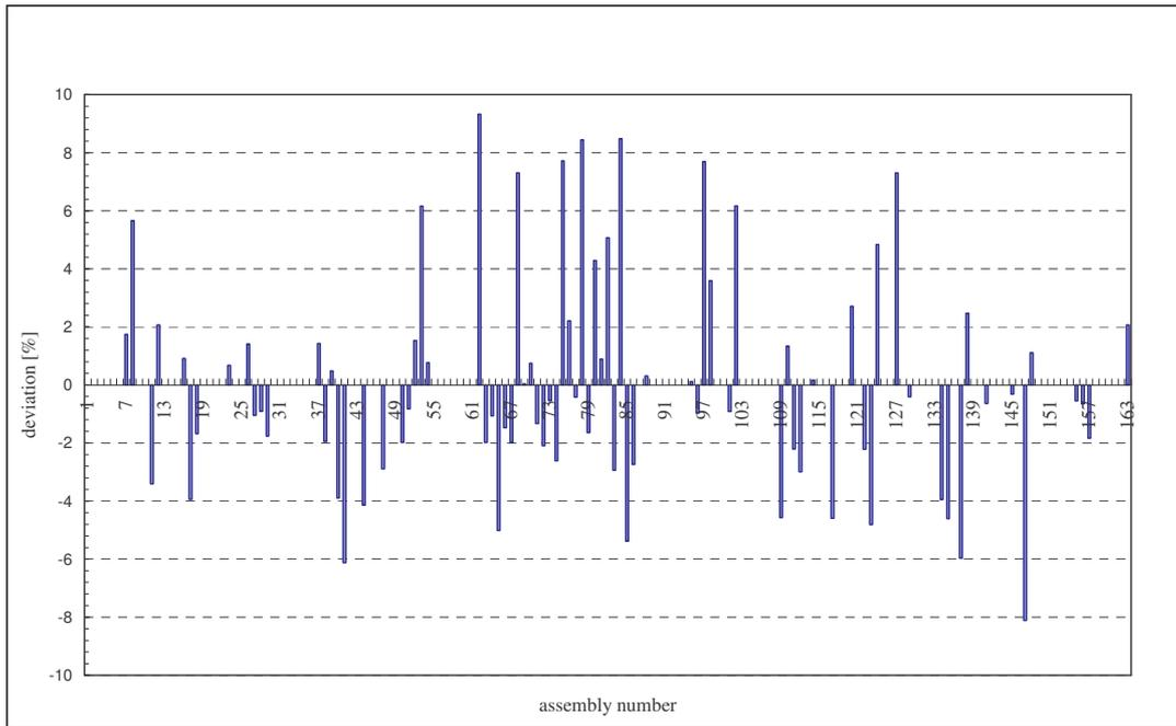
**Figure 6. State 1 - deviation of calculated central-pin power (method (3)) from measurement.**
