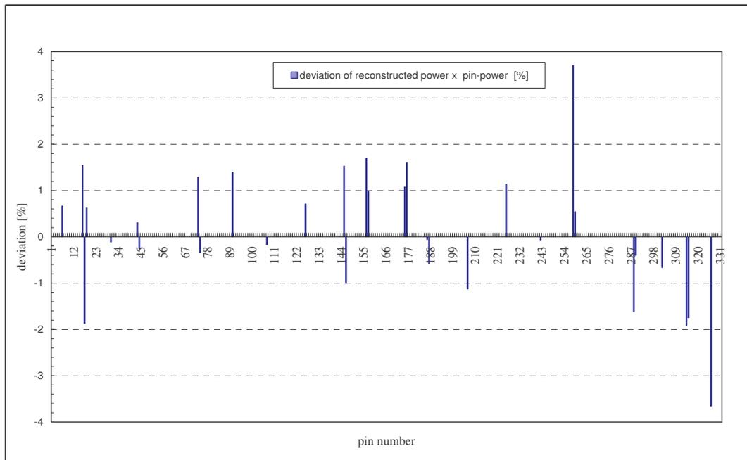
**Figure 5. State2 - deviation of calculated pin-power (method (3)) from measurement in fuel assembly No. 85.**
