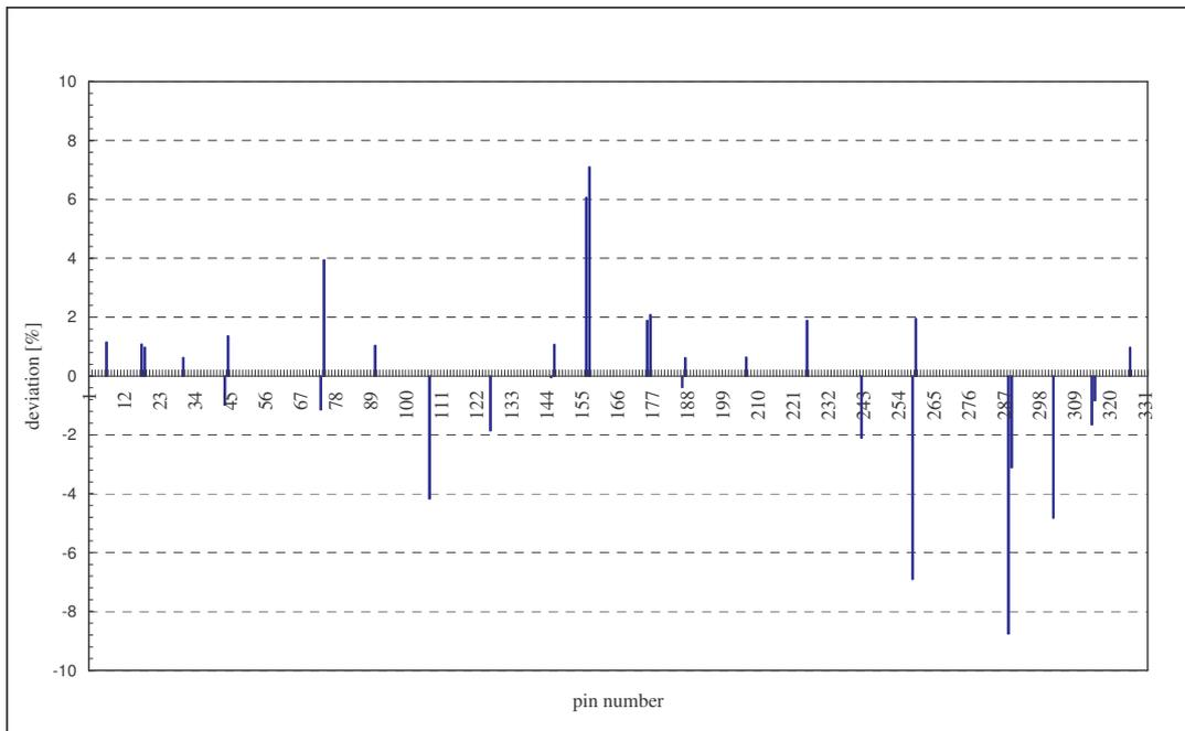
**Figure 7. State1 - deviation of calculated pin-power (method (3)) from measurement in fuel assembly No. 85.**
