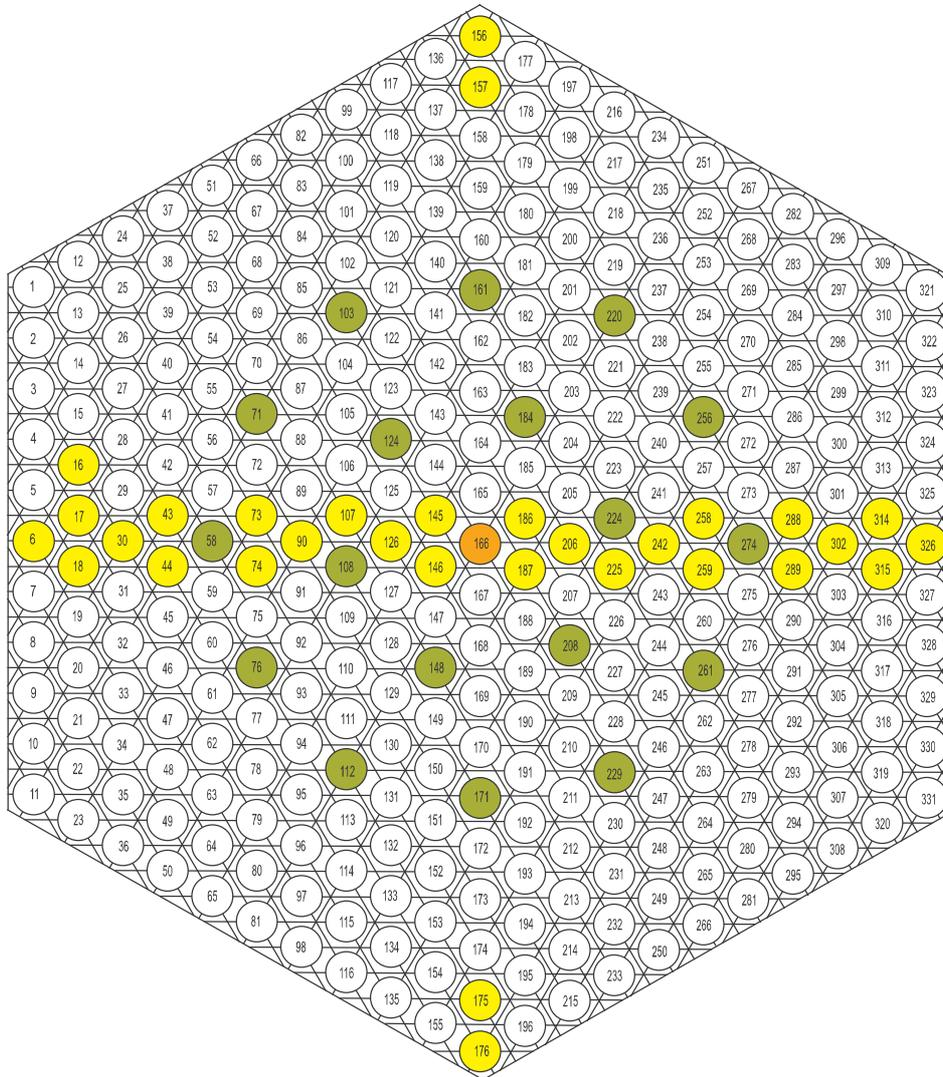
**Figure 4. Positions of measured pin powers (yellow) in fuel assembly No. 85. Green: positions of control rods (inserted in state 1, driven out in state 2). Orange (166): central tube. Pin No. 16 measured only in state 2.**
