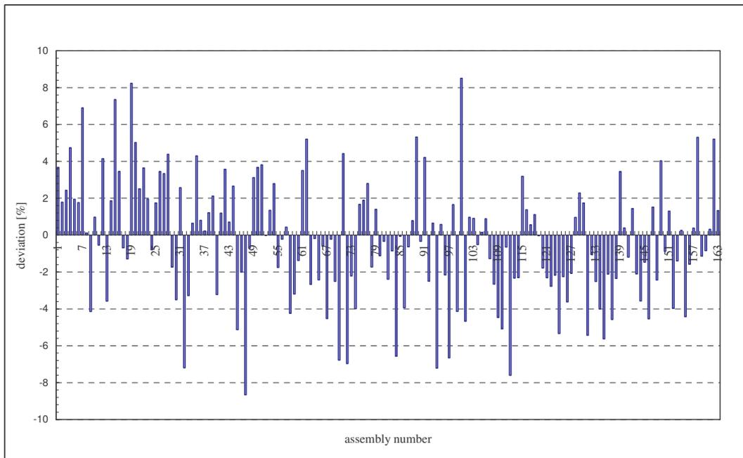
**Figure 3. State 2 – deviation of calculated central-pin power (method (3)) from measurement.**
