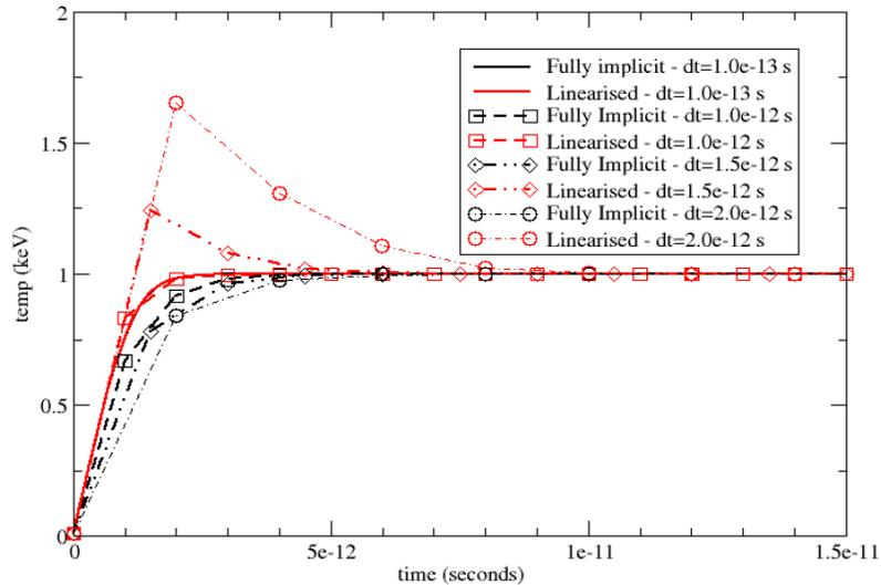
**Fig. 1. Study of the effect of linearization on the heating rate in an infinite medium. For large time-steps the temperature obtained from solving the linearized equations overshoots the equilibrium value and the material then has to cool into equilibrium. The fully implicit solution never overshoots, but does tend to overestimate the amount of thermal emission and is therefore less accurate than the linearization scheme for small enough time-steps.**
