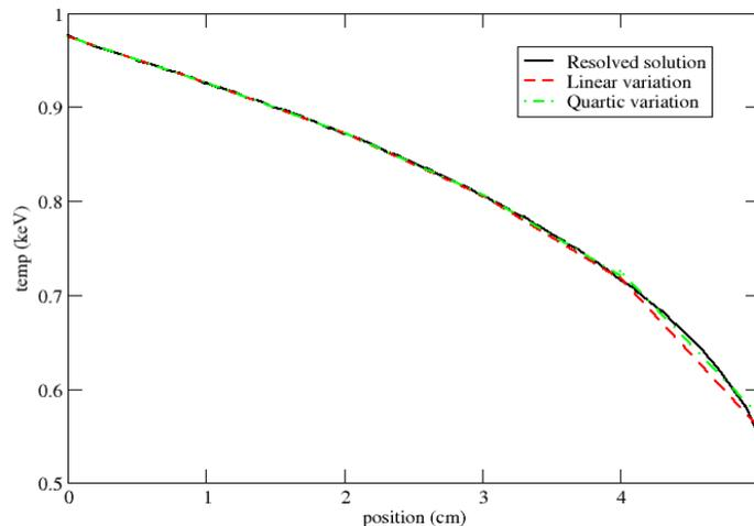
**Fig. 2. Comparison of the steady-state solutions for radiation flow through a 5 mean free path thick slab. Here we compare a converged 50 zone solution with 5-zone solutions obtained for the multiple linear scheme (temperature and blackbody energy density both linear) and the consistent linear scheme.**
