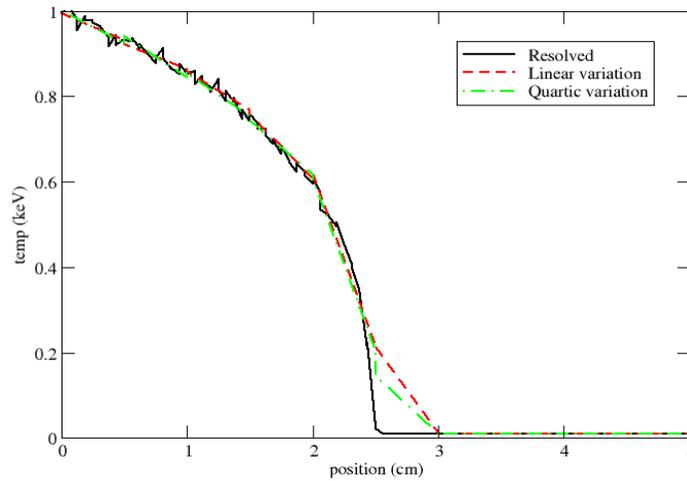
**Fig. 4. Comparison of the scheme for the Marshak wave problem at  $3 \times 10^{-7}$  seconds after the drive is applied. Here we compare the solutions obtained with 10 cells (100 mean free paths per cell) with the converged 80 cell (12.5 mean free paths per cell) solution.**
