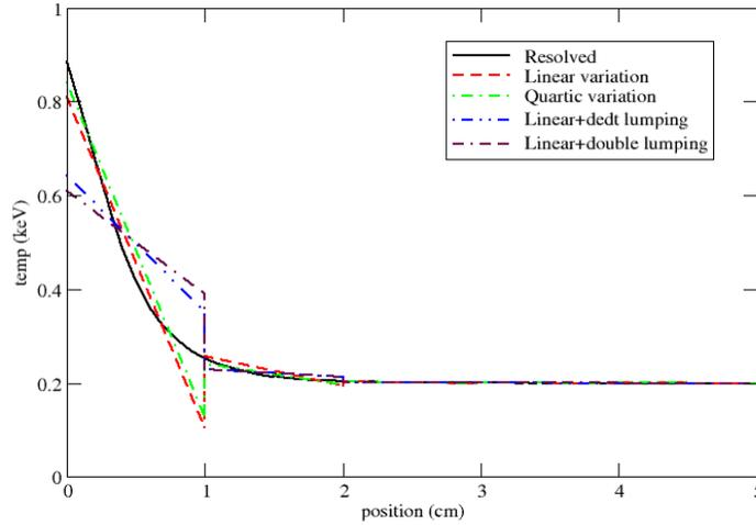
**Fig. 3. Comparison of the different lumping schemes applied to a time dependent problem. Here the slab is 10 mean free paths thick and starts in thermal equilibrium at 0.2 keV, heated by a 1 keV blackbody source at the left hand end. These results were generated with a time-step of  $10^{-11}$  seconds and the results are plotted at a time of  $3.5 \times 10^{-10}$  seconds after the drive is applied.**
