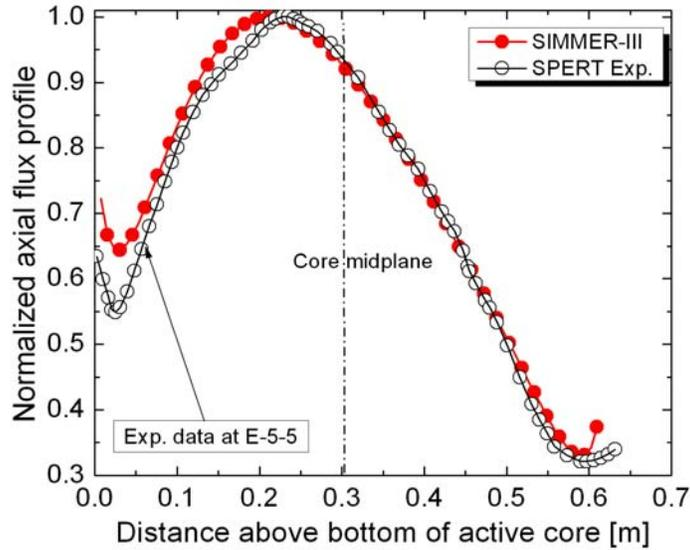
**Figure 7. Normalized axial neutron flux profile at the core center.**
