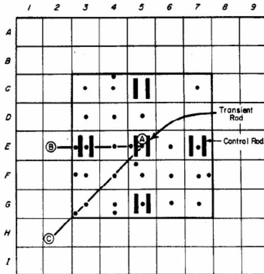
**Figure 6. Flux wire activation positions (Ref. 11).**
