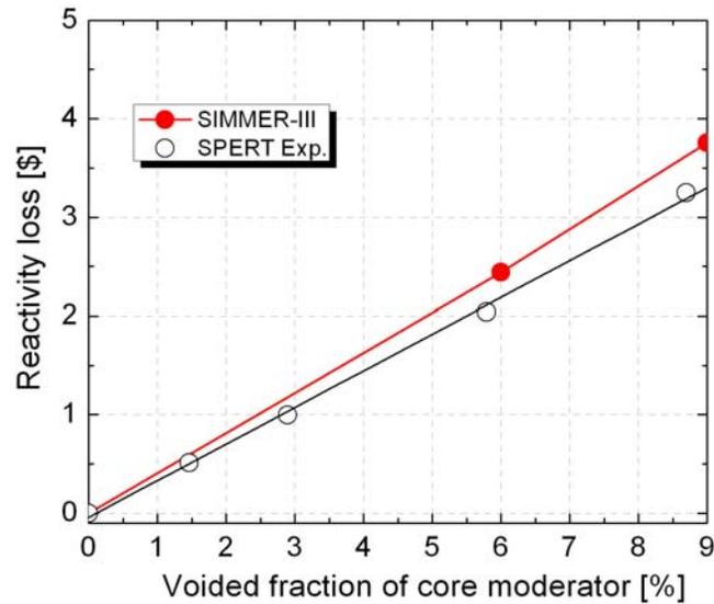
**Figure 9. Reactivity loss as a function of void fraction for a uniform distribution of voids.**
