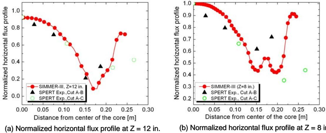
**Figure 8. Normalized horizontal neutron flux profiles at specified axial position. Half-width of the rectangular core is about 0.19 m.**
