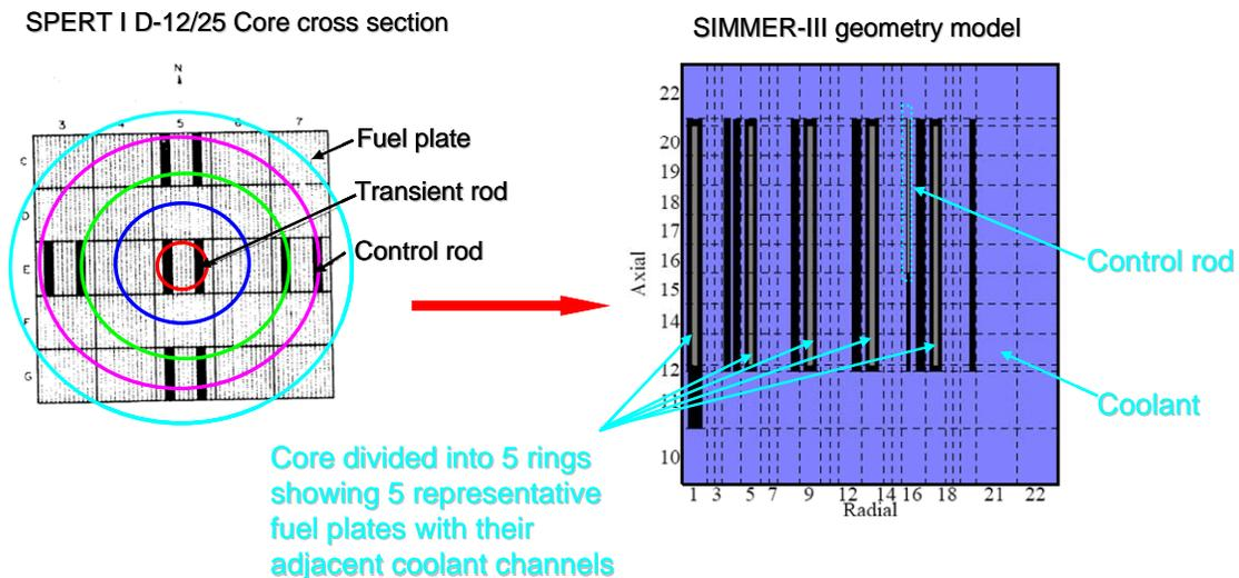
**Figure 4. Geometrical model of the SPERT I D-12/25 core in the SIMMER-III simulation.**
