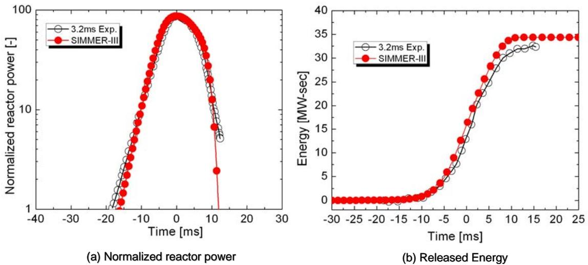
**Figure 10. Transients of the normalized reactor power and the released energy.**
