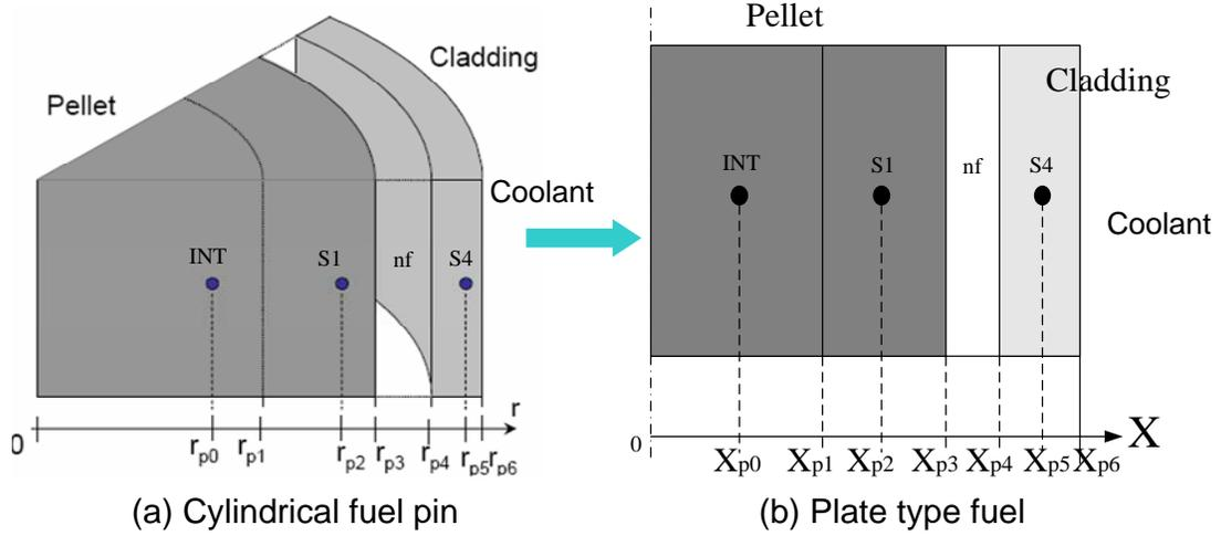
**Figure 1. Fuel pin configurations in SIMMER-III.**
