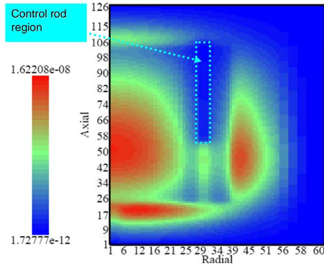
**Figure 5. Neutron flux distribution in the core represented by that of the 40<sup>th</sup> energy group.**
