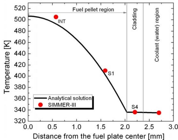
**Figure 2. Comparison of the X-direction temperature profile. INT, S1, S4 are the three nodes defined for the fuel plate in SIMMER-III (see Fig. 1).**
