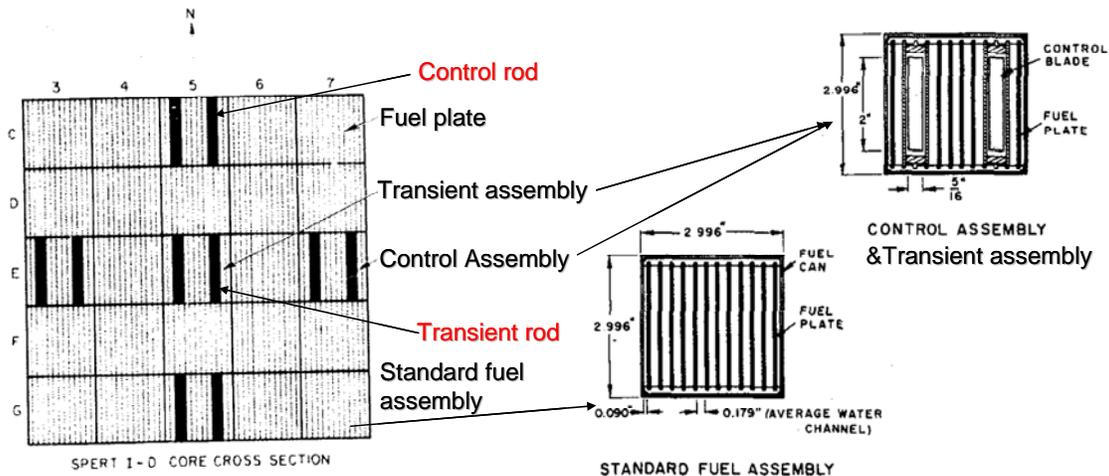
**Figure 3. A cutaway view of the SPERT I D-12/25 core cross section and the view of the fuel, control, and transient assemblies (Ref. 11).**
