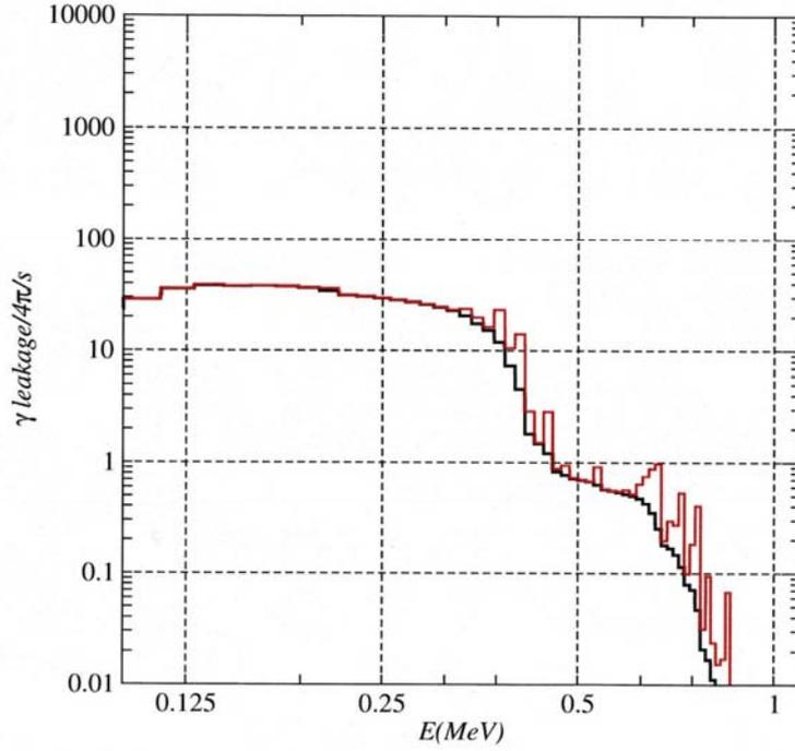
**Figure 1. Example of total (collided plus uncollided) multigroup  $\gamma$  leakage spectra (red) and collided only component (black)**
