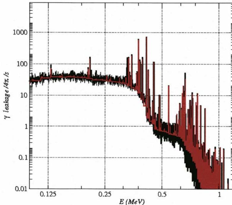
**Figure 4. Comparison of SGRD (red) and MCNP5 (black) calculated spectra for the water reflected sphere of plutonium nitrate solution test problem.**
