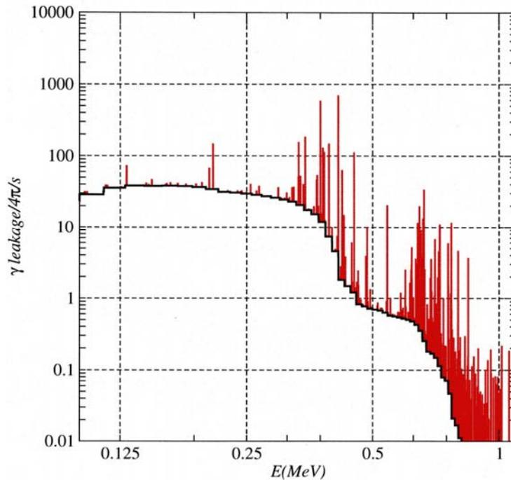
**Figure 2. Example of SGRD calculated spectra with multigroup scattered background and point-wise gamma lines.**
