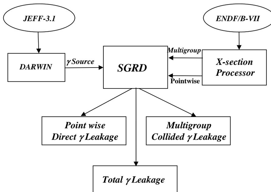
**Figure 3. SGRD input/output flow diagram.**
