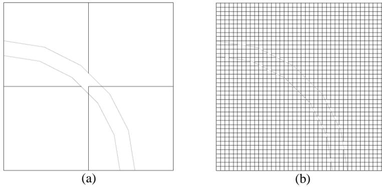
**Figure 2. Pin Cell Mesh Structures considered in the sensitivity analysis.**
