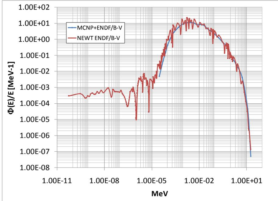
**Fig. 5. MCNP, NEWT calculated neutron energy spectra**
