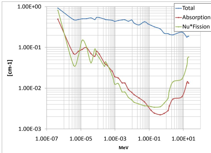
**Fig. 7 Homogenized macroscopic cross sections with ENDF/B-V**
