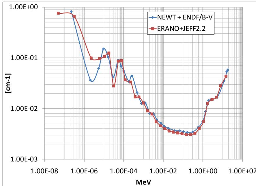
**Fig. 9 NEWT-to-ERANOS  $\nu\Sigma_f$  homogenized macroscopic cross sections comparison**
