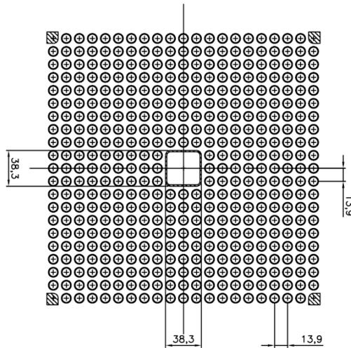
**Figure 1. Fuel Assembly Design**
