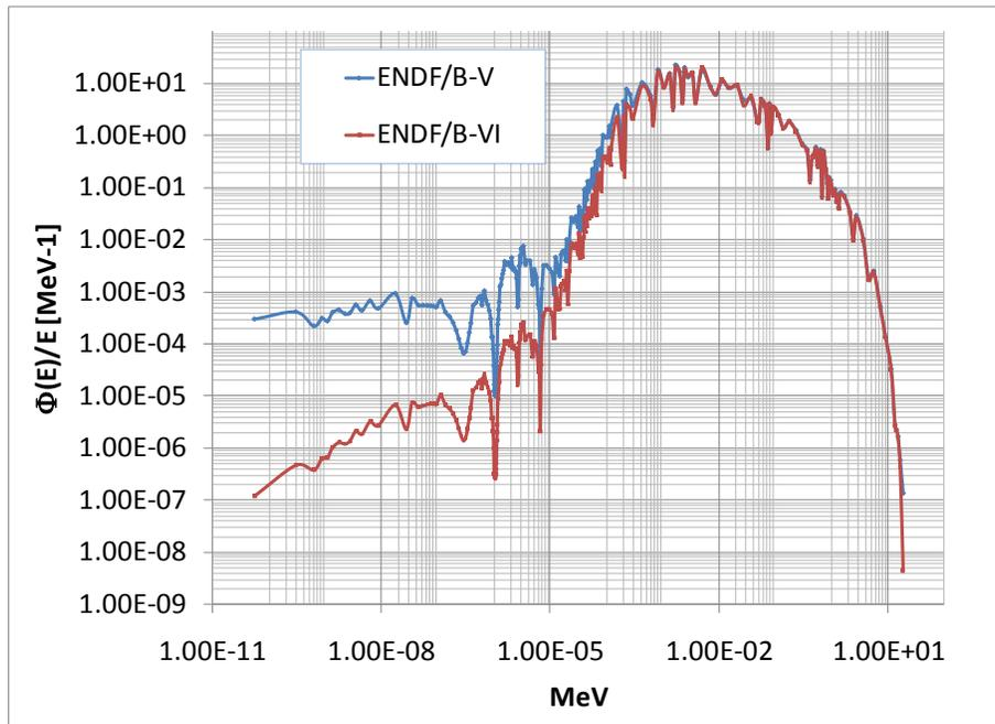
**Figure 4. Neutron Flux Energy spectrum**
