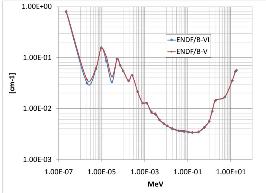
**Fig. 8 NEWT  $\nu\Sigma_f$  homogenized macroscopic cross sections calculated with ENDF/B-V,VI**
