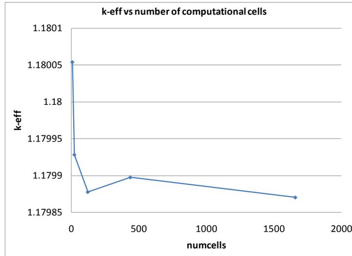
**Figure 3. Effective k as a function of mesh size**
