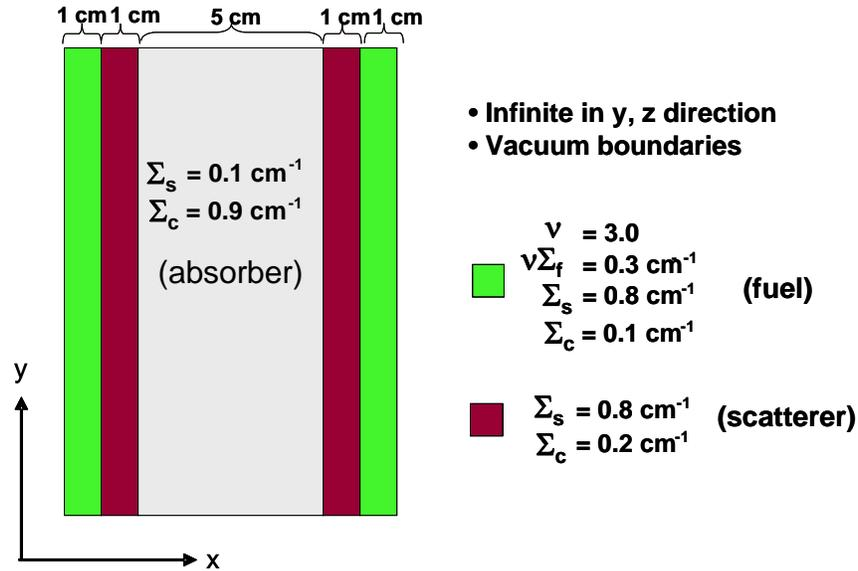
Figure 2: Makeup of 1-D inhomogeneous slab problem
