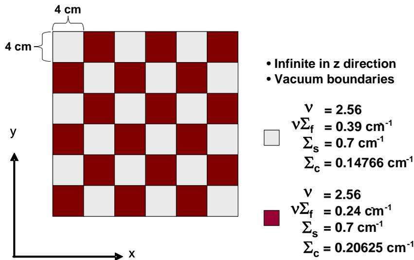
Figure 1: Makeup of 1-D inhomogeneous slab problem
