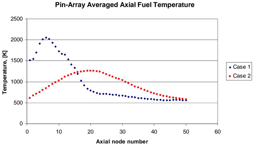
**Figure 6. Axial Fuel Temperature Distributions for Case 1 and 2**
