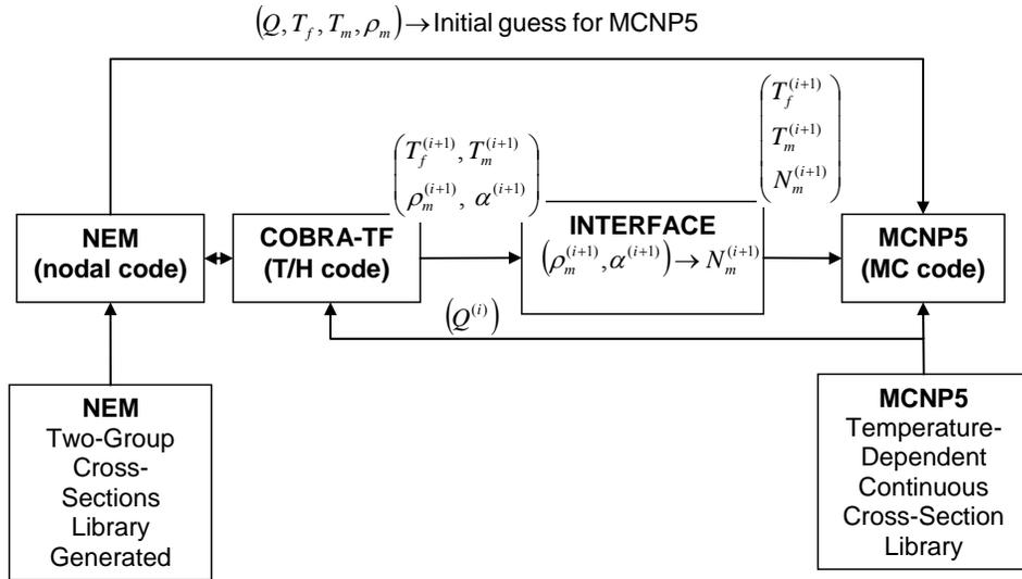
Figure 1. Multi-level NEM/MCNP5/CTF coupling scheme
