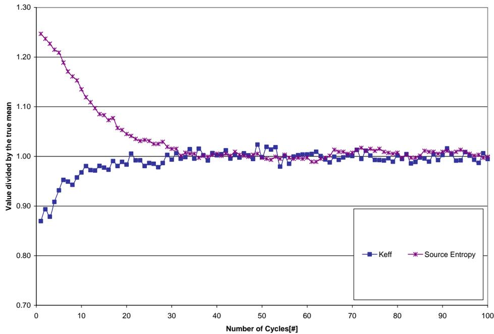
**Figure 4.  $k_{\text{eff}}$  and Shannon Entropy convergence for 3-D BWR 2x2 fuel-pin array**
