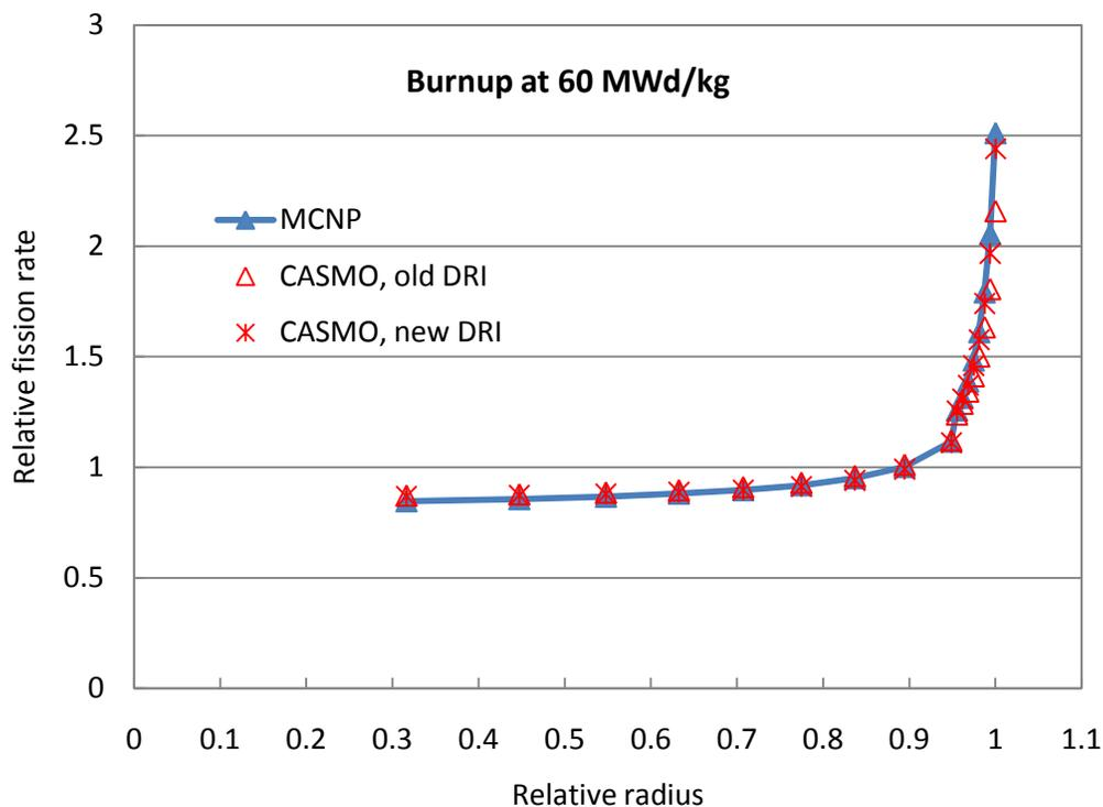
**Figure 3. Fission rate comparison at 60 MWd/kg.**
