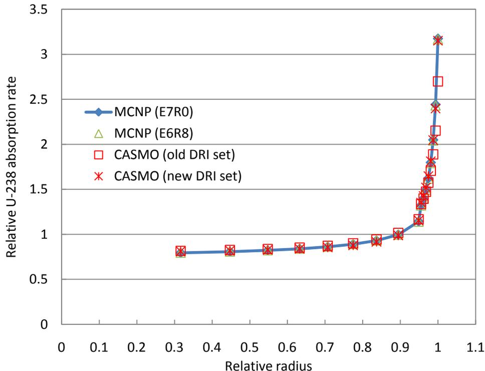
**Figure 2. U-238 absorption rate distribution at BOL.**
