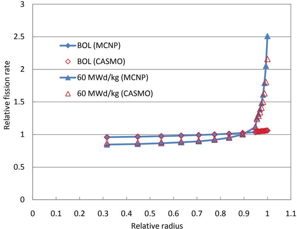
**Figure 1. Fission rate comparison between CASMO-5 and MCNP-5.**
