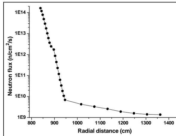
**Figure 5. Neutron flux distribution in the mid-plane port**
