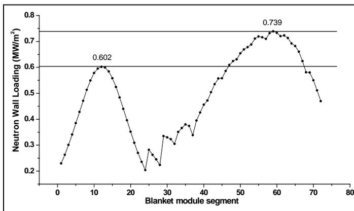
**Figure 1. The distribution of neutron wall loading on the first wall**
