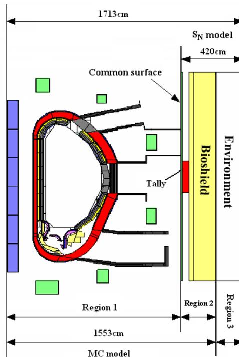
**Figure 6. Processing of ITER benchmark model by RCAM**
