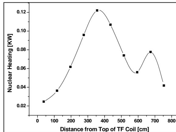
**Figure 3. Total TF coil heating in two inboard legs**
