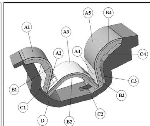
**Figure 2. Tally location on divertor cassette loading on the first wall**
