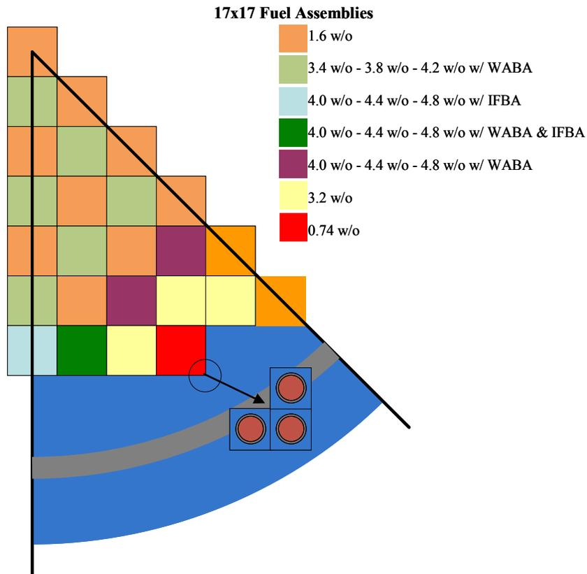
Figure 1. PWR Core Model Used in the Calculations
