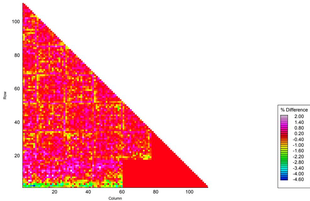
**Figure 3. Percent Difference in Relative Pin Power between MCNP and PARAGON Calculations**
