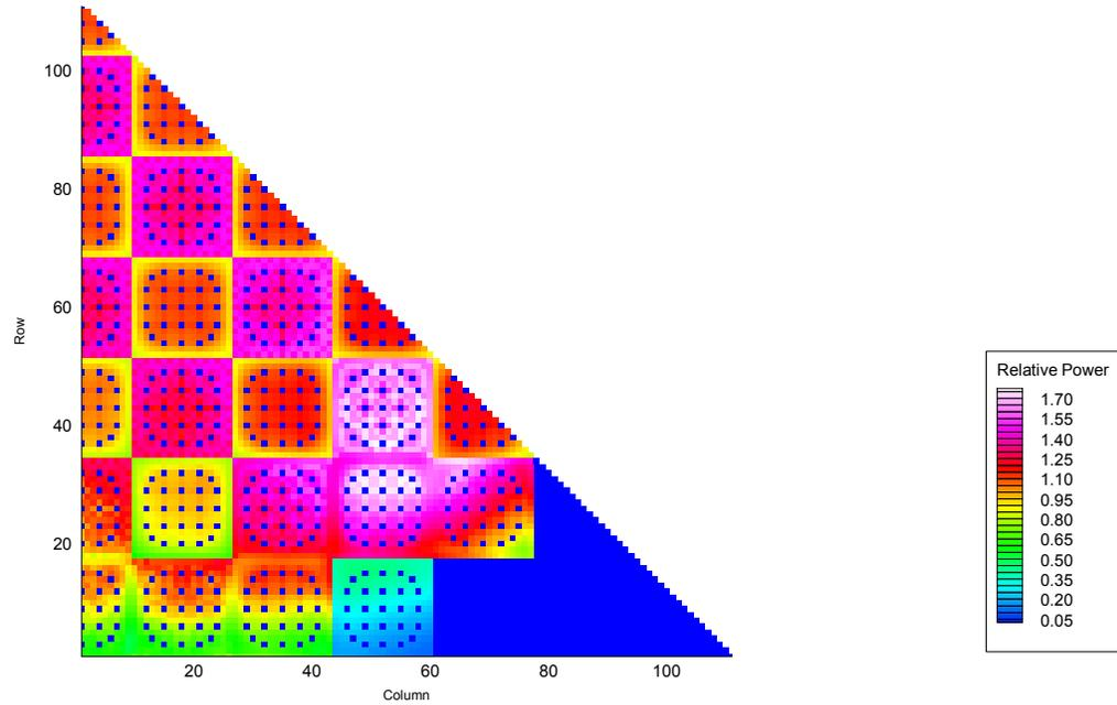
**Figure 2. Whole Core Relative Pin-Power Distribution as Calculated by PARAGON**
