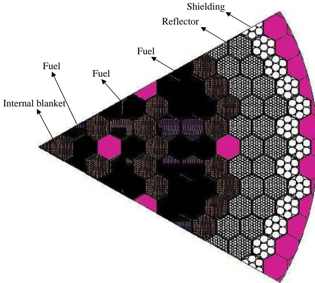
**Figure 2. MCNP5 generated schematic of the one-sixth symmetric core showing core regions, radial and axial blankets, shield, reflective and driver fuel assemblies**
