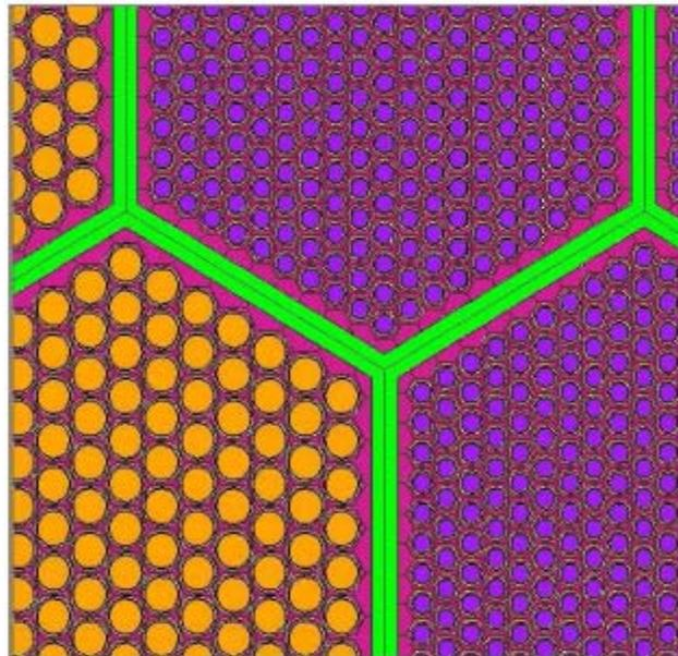
**Figure 3. A close up of the one-sixth core model depicting the difference in the size of pins between the driver fuel assemblies and blankets**
