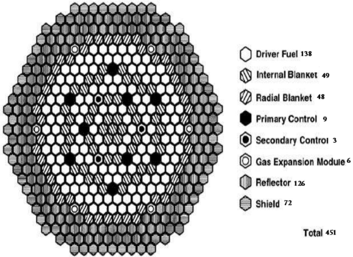
Figure 1. S-PRISM metal core configuration [8]
