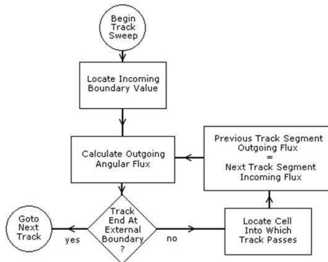
Figure 1: MOCK-3DK Track Sweep Procedure
