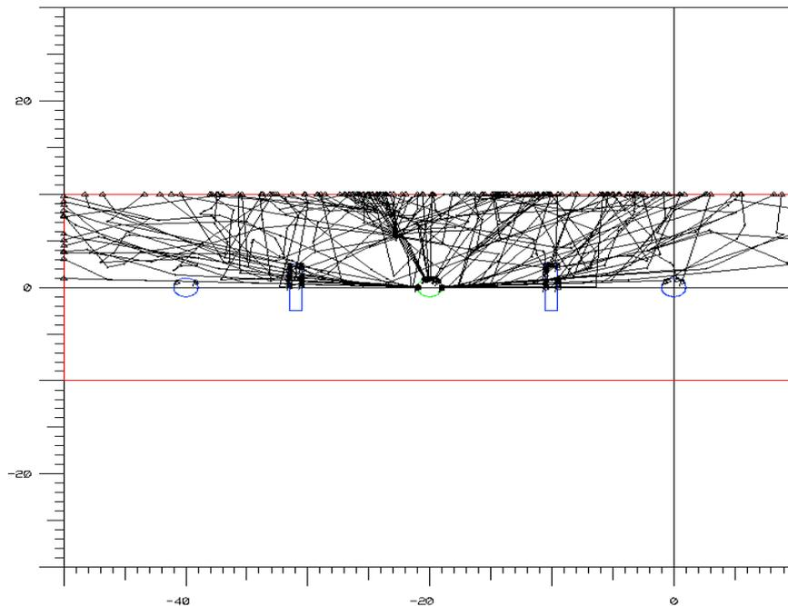
**Figure 5. The problem geometry and the first 50 neutron tracks when the original fix-up method is used with plastic shielding slabs**
