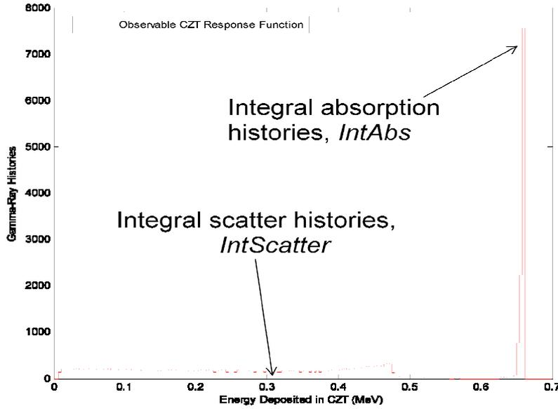
**Figure 2. Sample CZT spectrum obtained from MCNP-PoliMi collision output file after Compton suppression technique is performed.**
