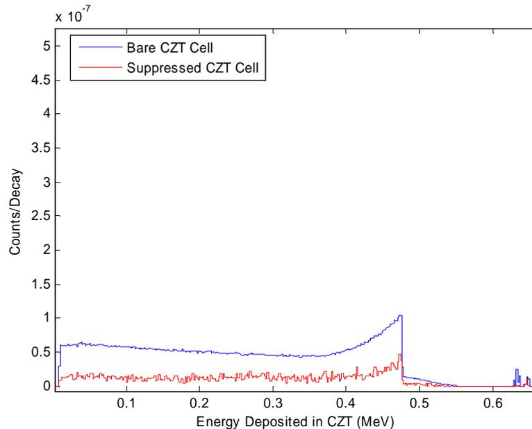
**Figure 3. Comparison of an optimized Compton suppression system with a bare CZT cell response to a  $^{137}\text{Cs}$  source.**
