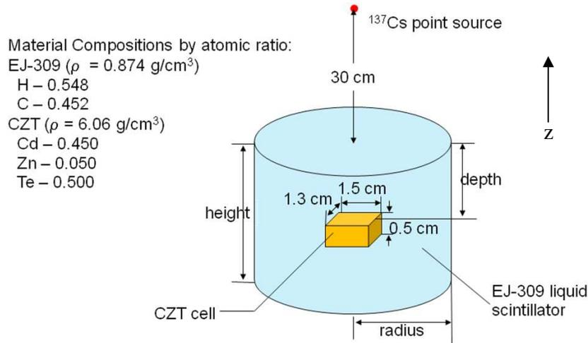
**Figure 1. MCNP-PoliMi model of a CZT/liquid scintillator Compton suppression system.**
