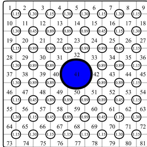
**Figure 1. Cross sectional view of the fuel bundle with subchannel indices and relative rod power listed [1]. The shaded rod in the center is a water rod and is not heated.**
