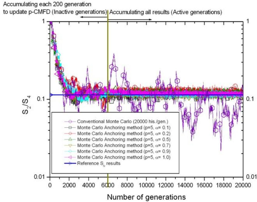
Figure 9. Fission source ratios versus various anchoring factors in test problem 2
