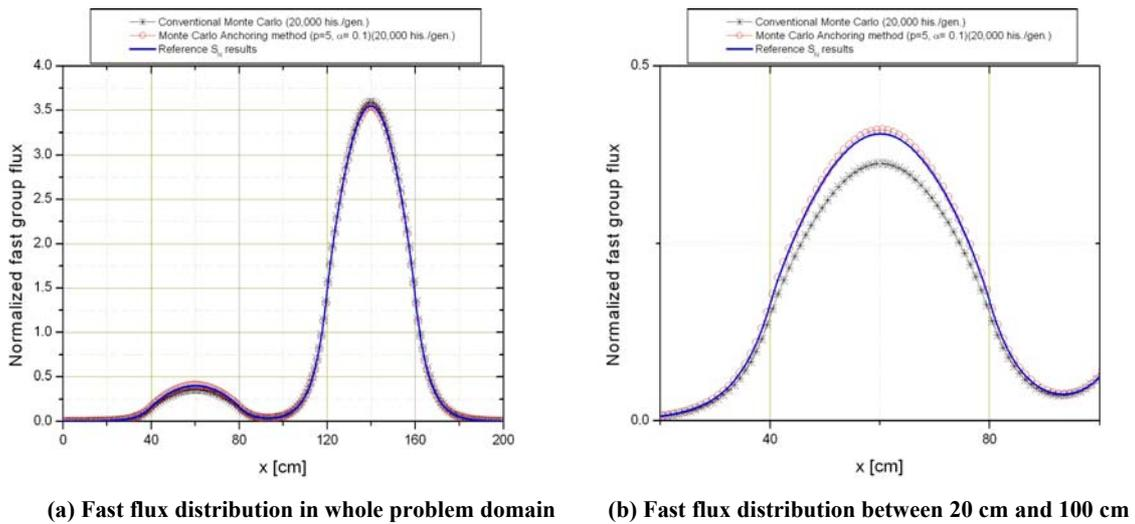
Figure 7. Normalized fast flux distributions of test problem 2
