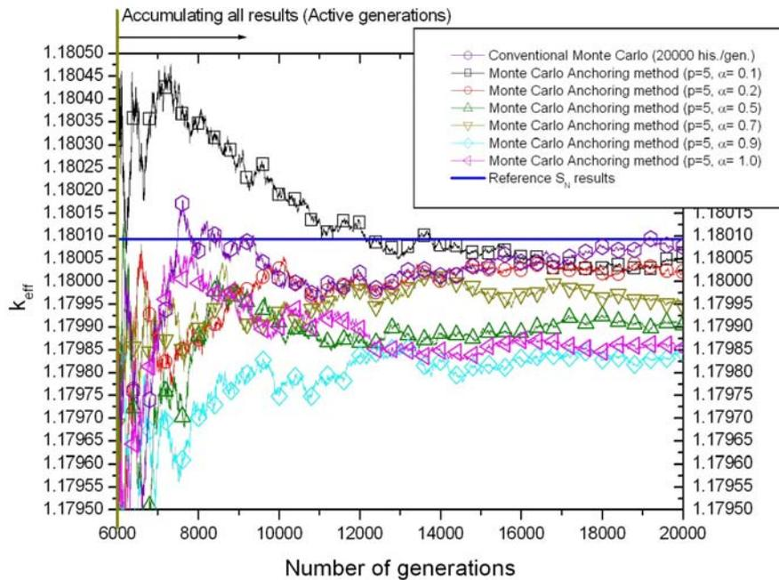
Figure 10.  $k_{eff}$  versus various anchoring factors in test problem 2
