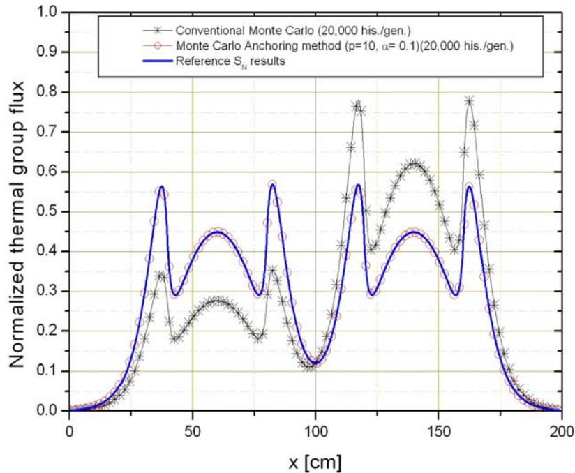
Figure 5. Normalized thermal flux distributions of test problem 1
