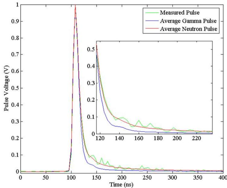
**Figure 5. Illustration of the average-pulses PSD method. Measured neutron pulse with average neutron and gamma-ray pulses are shown.**
