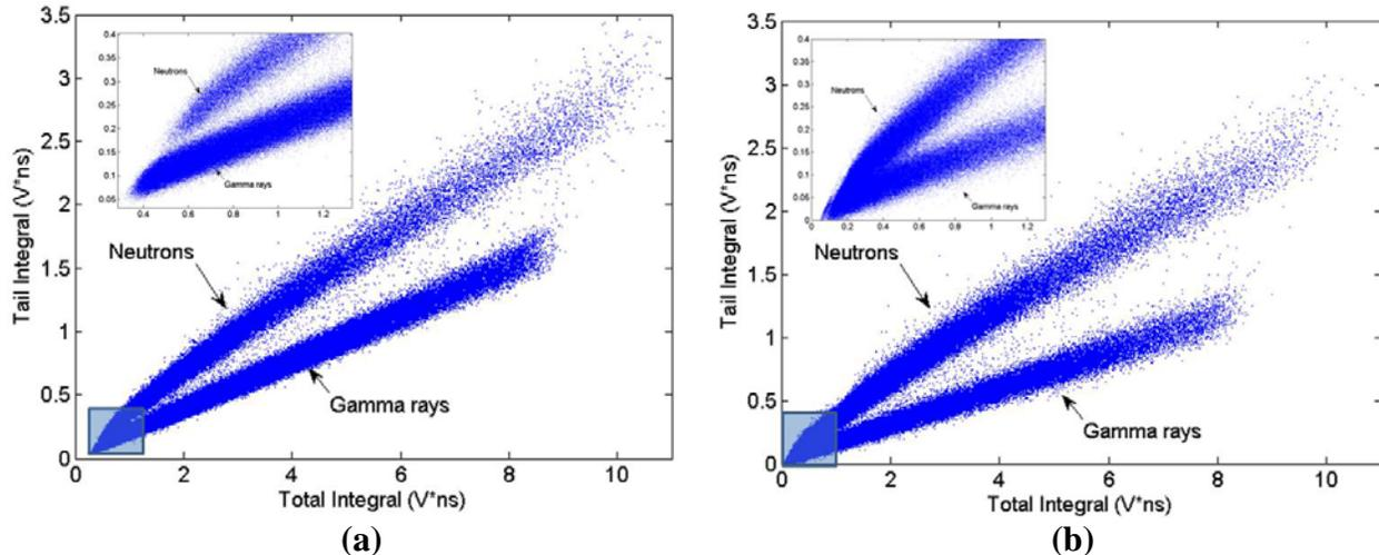
**Figure 4. Tail integral versus total integral for (a) 70 keVee threshold, (b): 26 keVee (200 keV neutron energy) threshold. Standard charge-integration PSD method was used.**
