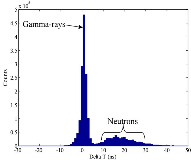
**Figure 2. Measured time-of-flight distribution from a Cf-252 source.**
