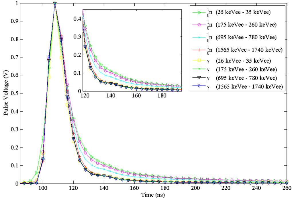
**Figure 3. Normalized average neutron and gamma-ray pulses (zoomed in view of the tails are inset to emphasize the differences). Large differences are observed between neutron pulses themselves and neutron and gamma-ray pulses.**
