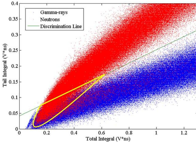
**Figure 6. Time-of-flight attributed neutron and gamma-ray pulses illustrate the shortcoming of the charge-integration method for small pulses (overlap region shown with the yellow marker).**
