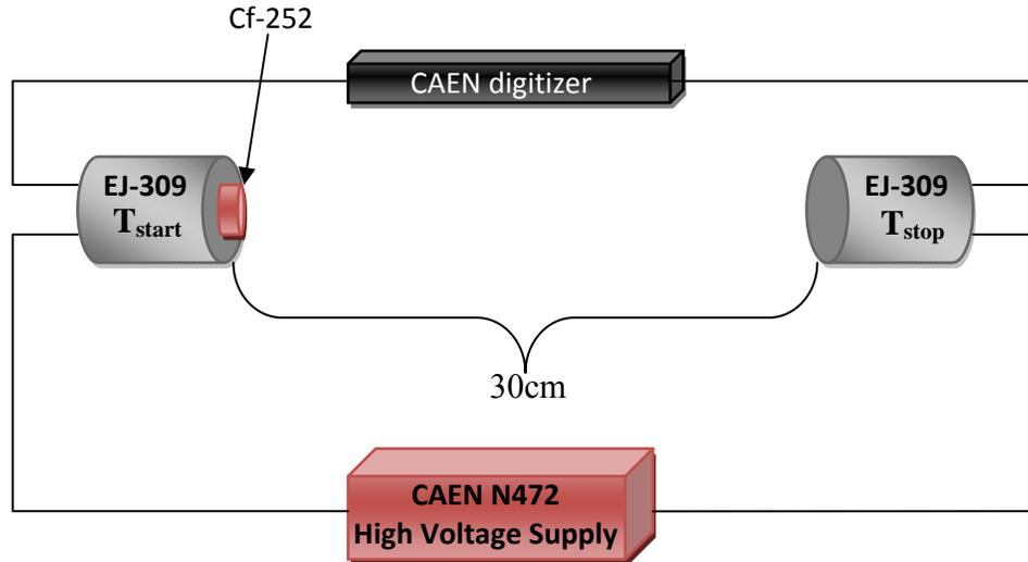
**Figure 1. TOF Measurement Setup**
