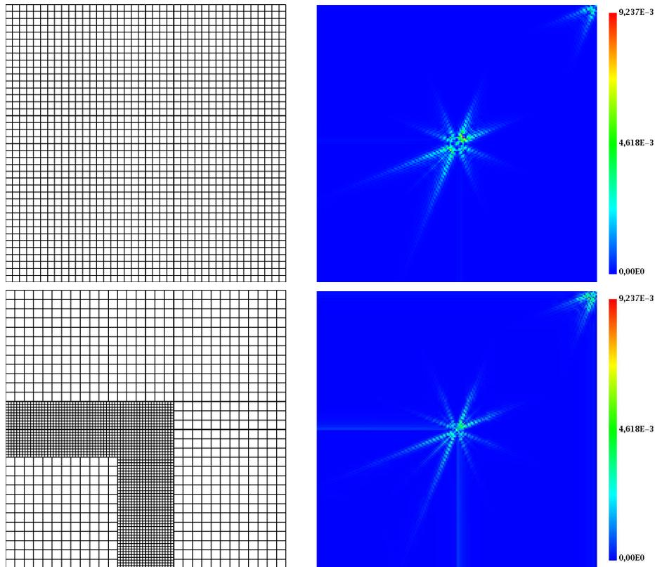
**Figure 5. Conforming and non-conforming meshes and relative cell wise errors**
