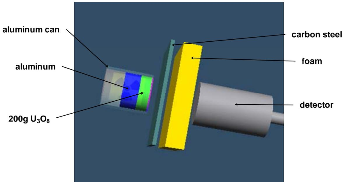
**Figure 1. Test geometry 1: aluminum cylinder on end containing uranium oxide with foam and carbon steel shielding. The free parameters include combinations of the source matrix density, source matrix fill height, aluminum container wall thickness, and carbon steel shielding thickness.**
