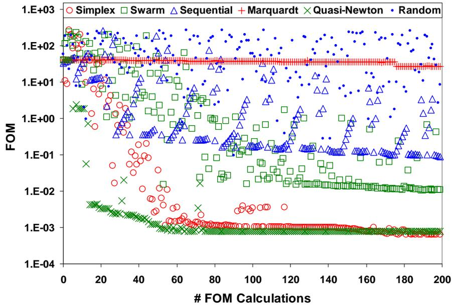
**Figure 6. Optimization progression for Geometry 2 Test 1 (modeled), with four free parameters: uranium solution density, uranium solution fill height, polyethylene container wall thickness, and container radius.**
