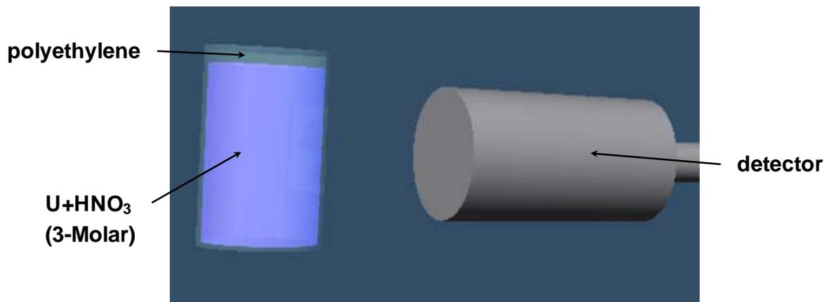
**Figure 3. Test geometry 2: polyethylene cylinder from the side filled with a solution of uranium in nitric acid. The free parameters included combinations of source matrix density, source matrix fill height, cylinder radius, and container wall thickness.**
