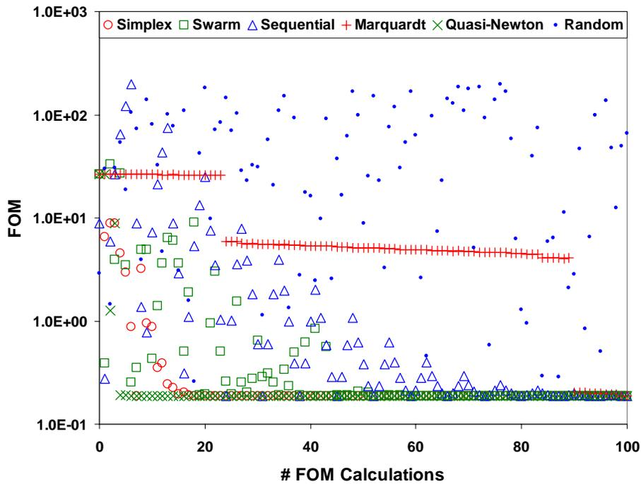
**Figure 5. Optimization progression for Geometry 1 Test 2 (measured), with only one free parameter: steel shielding thickness. The actual thickness was set to 7 mm with the minimum bound at 4 mm and maximum bound at 15 mm.**
