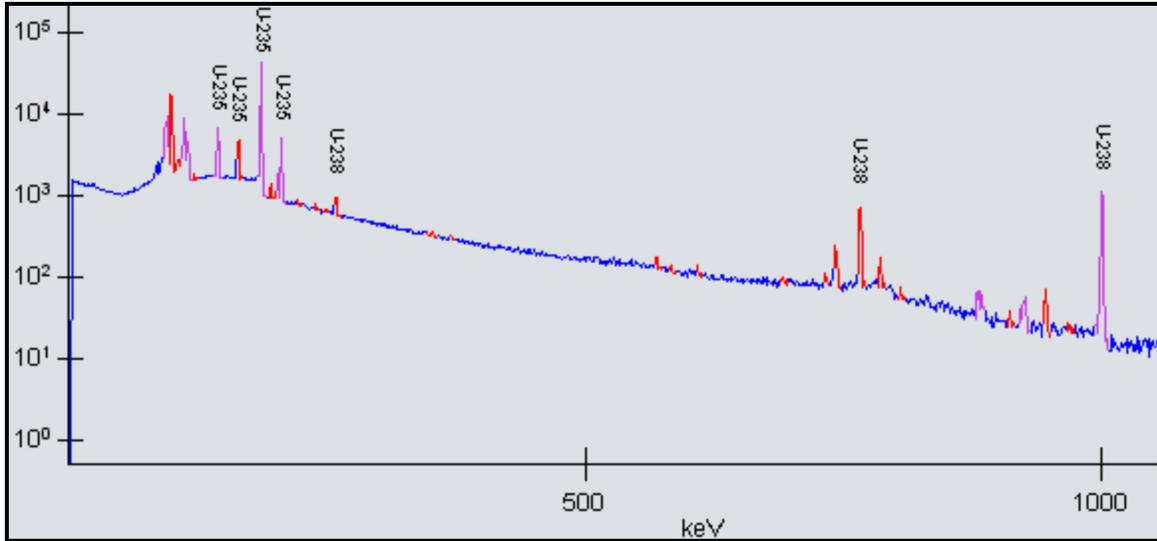
**Figure 2. Measured spectrum acquired for geometry 1, with 3 photopeak lines associated with <sup>238</sup>U (258, 756, and 1001 keV) and 4 photopeak lines associated with <sup>235</sup>U (144, 163, 186, and 205 keV).**
