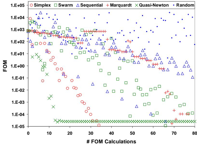
**Figure 4. Optimization progression for Geometry 1 Test 2 (modeled), with only one free parameter: steel shielding thickness. The actual thickness was set to 7 mm with the minimum bound at 4 mm and maximum bound at 15 mm.**
