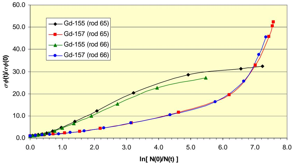
**Figure 20. Relative change in gadolinium reaction rates as functions of the natural logarithm of concentration ratios**
