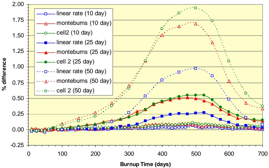
Figure 15. Percent Difference in  $^{149}\text{Sm}$  Concentrations Relative to Reference Depletion
