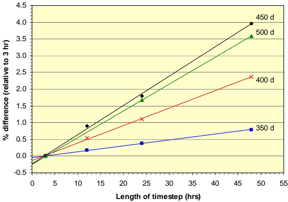
Figure 3. Convergence analysis of  $^{157}\text{Gd}$  concentrations with constant flux depletions showing projected error of 3-hour solutions at various burnup times
