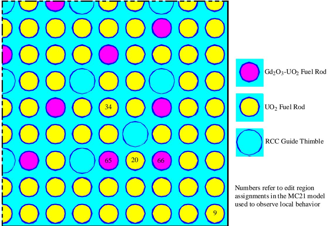
Figure 1. Geometry laydown of PWR quarter-assembly
