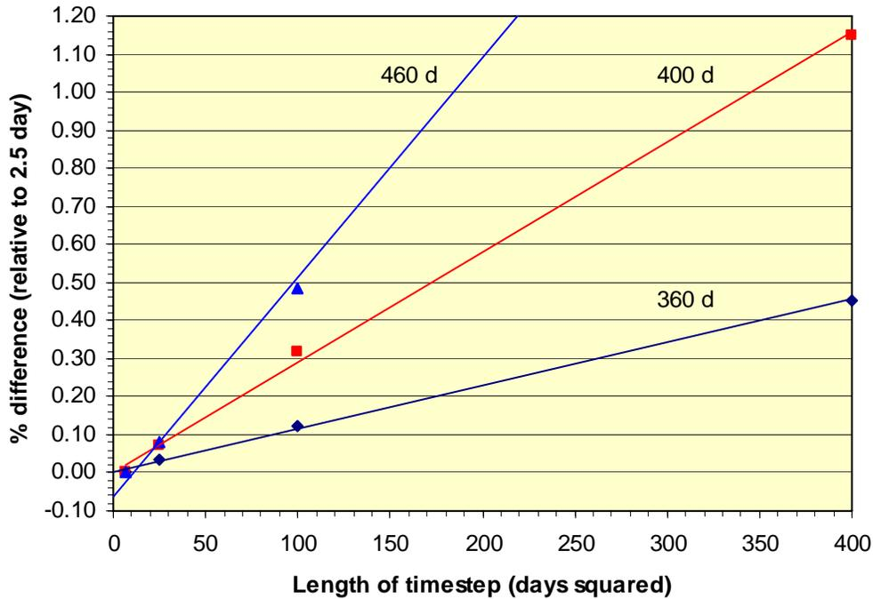
**Figure 5. Convergence analysis of  $^{157}\text{Gd}$  concentrations with *linear rate* depletions showing projected error of 2.5-day solutions at various burnup times**
