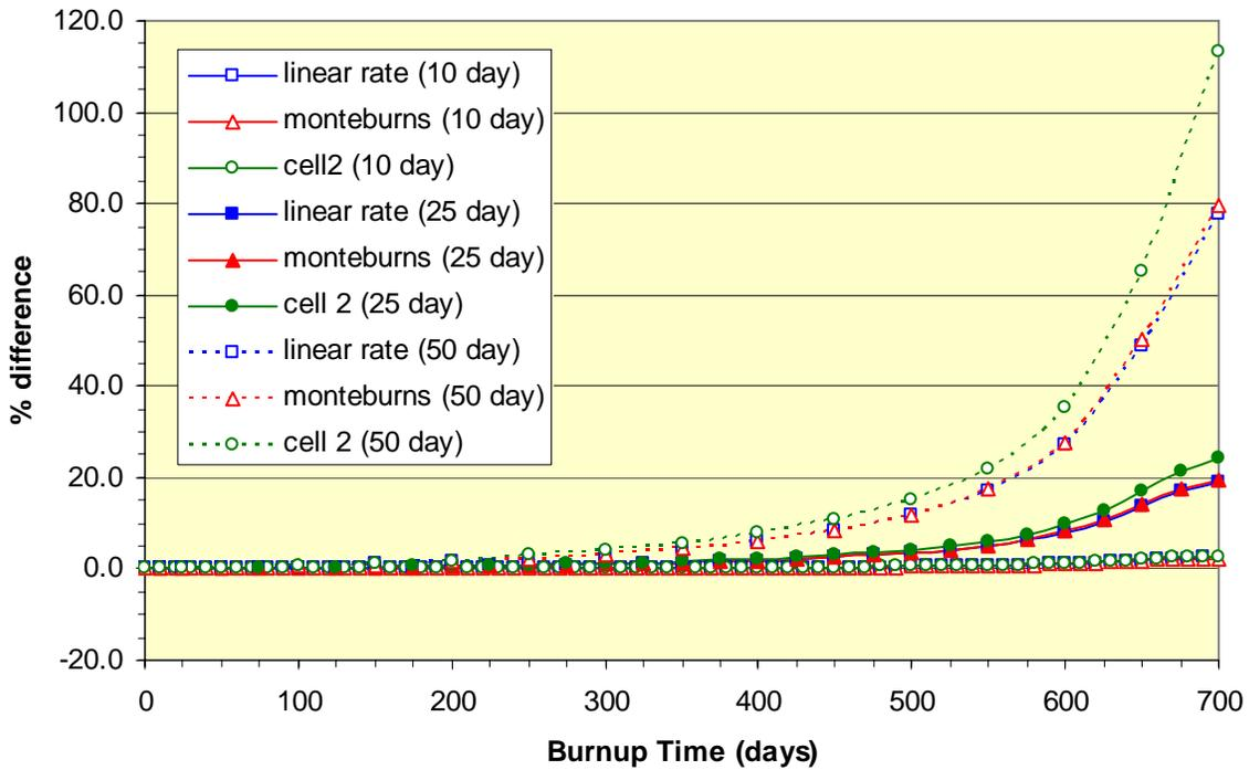
Figure 18. Percent difference in <sup>155</sup>Gd concentrations when using 10-region Gd-U fuel rods
