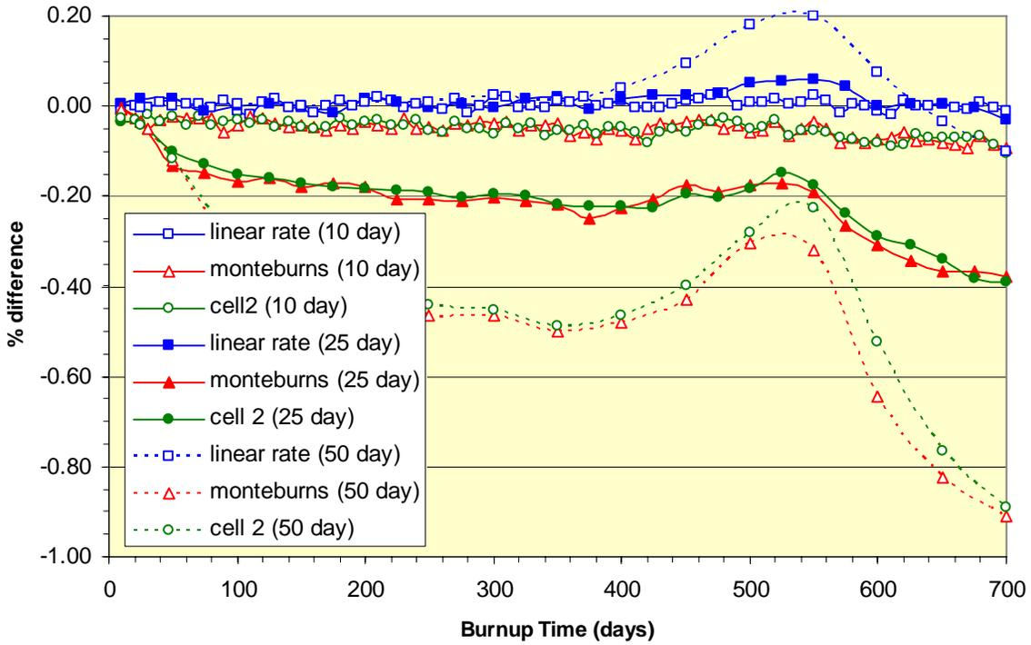
Figure 14. Percent Difference in  $^{149}\text{Pm}$  Concentrations Relative to Reference Depletion
