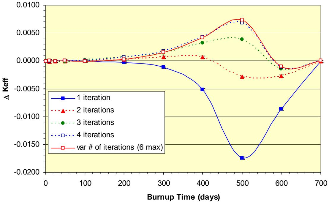
Figure 21. Change in keff as a result of iterating on the predictor-corrector steps
