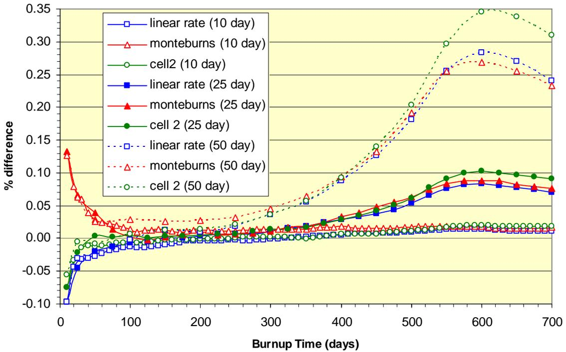
Figure 10. Percent Difference in  $^{239}\text{Pu}$  Concentrations Relative to Reference Depletion
