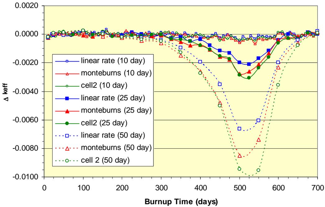
**Figure 6. Difference in  $k_{eff}$  relative to the reference *linear rate* depletion (maximum size of timestep in parentheses)**
