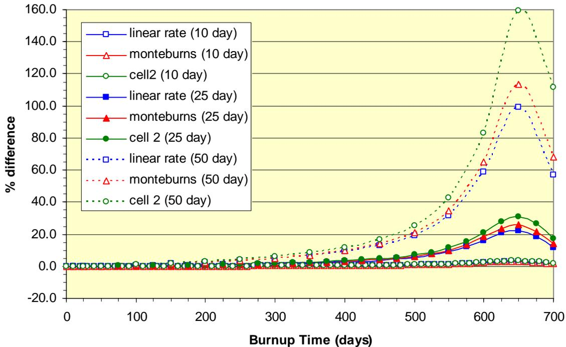
Figure 19. Percent difference in  $^{157}\text{Gd}$  concentrations when using 10-region Gd-U fuel rods
