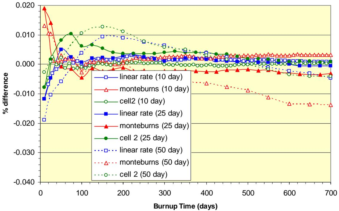
Figure 12. Percent Difference in the Fission Counter Relative to Reference Depletion
