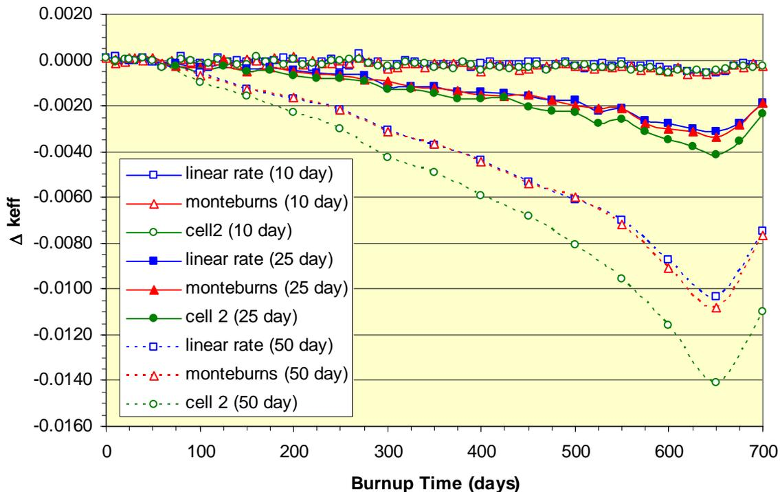
**Figure 16. Difference in  $k_{\text{eff}}$  relative to the reference *linear rate* depletion using 10-region Gd-U fuel rods**
