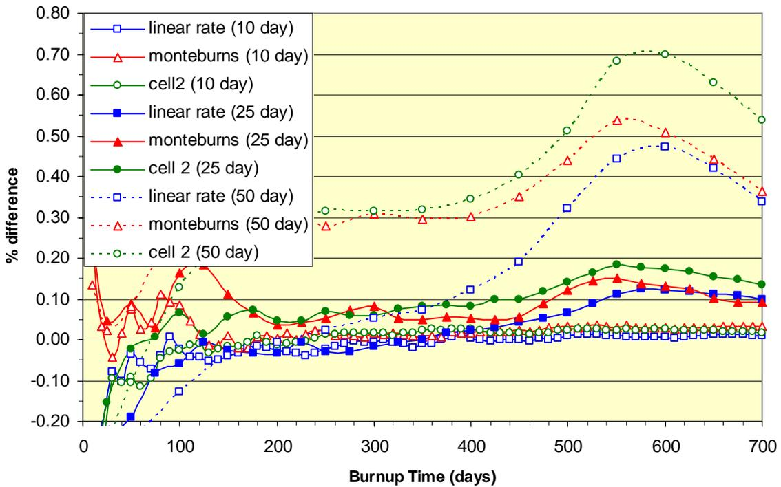
Figure 11. Percent Difference in  $^{241}\text{Pu}$  Concentrations Relative to Reference Depletion
