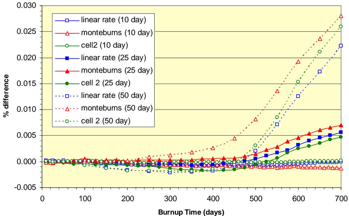
Figure 9. Percent Difference in  $^{235}\text{U}$  Concentrations Relative to Reference Depletion
