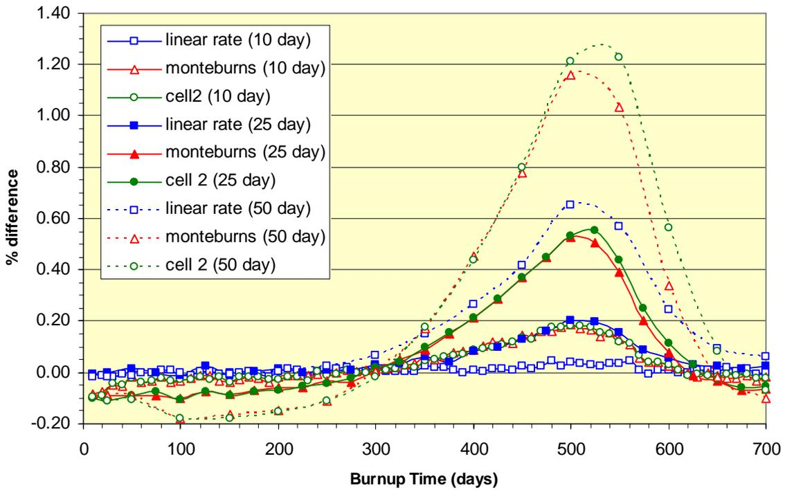
Figure 13. Percent Difference in <sup>135</sup>Xe Concentrations Relative to Reference Depletion
