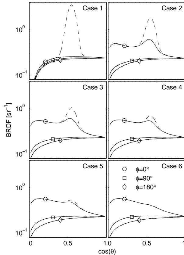
**Figure 5.** Comparison of BRDF results computed directly with CASIO-DISORT and with the ISBRDF package. Cases 1 through 6 correspond to snow layer thicknesses of 0 (bare ice), 0.5, 1, 1.5, 2, and 3 mm, respectively.
