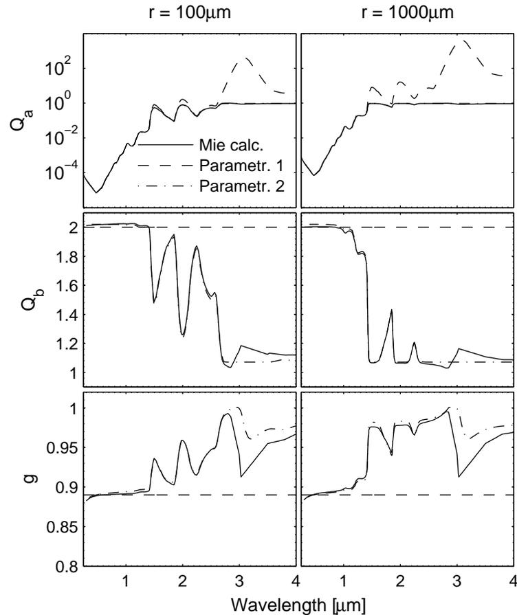
**Figure 1.** Comparisons of IOPs calculated using Mie theory with those obtained using Parameterization 1, which is valid for wavelengths shorter than about  $1.2 \mu\text{m}$  [9], and Parameterization 2, which is valid also in the near infrared.
