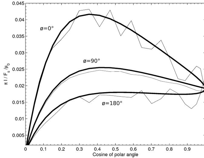
**Figure 2.** Comparisons of radiance computations done with (thick lines) and without (thin lines) use of the reduced forward scattering transformations for a slab of ice of thickness  $h = 1$  m. Here  $g_{max}$  was set to 0.9, which for  $\tau = 500$  ( $b = 490 \text{ m}^{-1}$  and  $a = 10 \text{ m}^{-1}$ ) and  $g = 0.99$ , gives  $\tau' = 59$  and  $1 - \omega' = 0.17$ .
