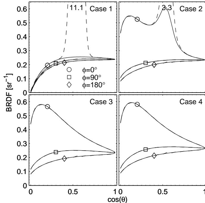
**Figure 4.** Same as Fig. 3 but now with the Gaussian specular reflection component (FWHM = 5°) included in ISBRDF. The numbers written on the Gaussian peak indicate its maximum value.
