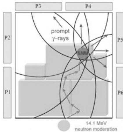
**Figure 5. Slow fission event: a thermal neutron captures on U-235, resulting in 4-fold gamma ray coincidences in adjacent panels P3, P4, P5, and P6. The location of SNM is determined from the relative nanosecond timing of gamma rays in the LKr detectors [18].**
