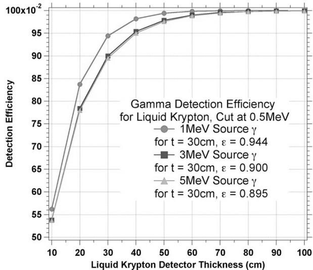
**Figure 2. Simulation of liquid krypton detector efficiency using MCNP.**
