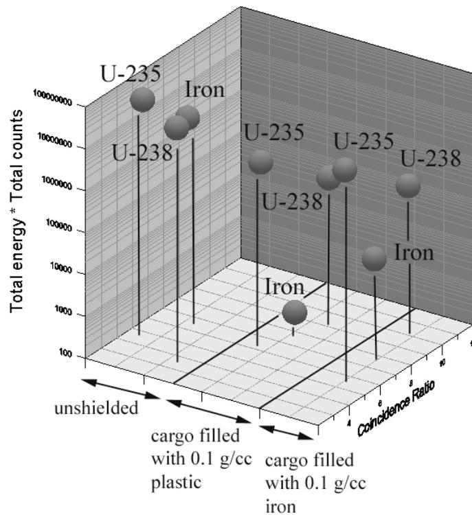
**Figure 6. Hyperspace for SNM detection in bare cargo, cargo filled with plastic, and cargo filled with iron.**
