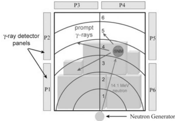
**Figure 4. Fast fission event: a 14.1 MeV neutron initiates fission in SNM to produce a multi-gamma jet resulting in 3-fold coincidences in adjacent panels P1, P2, and P3 in coincidence with the alpha detector [18].**
