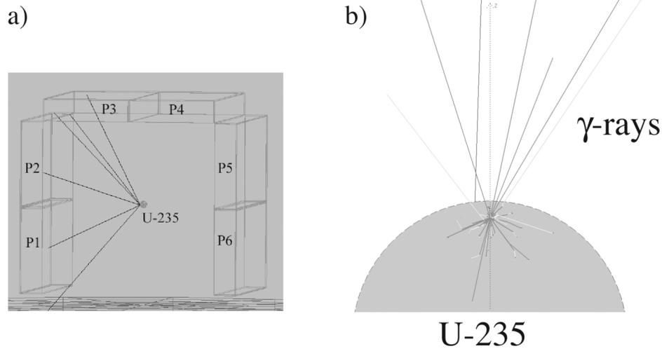
**Figure 3. a) Coincidence event in detector panels P1, P2, and P3 due to prompt gamma rays from neutron-induced fission of U-235. The gamma rays escape in a “jet structure” due to self-attenuation of gamma rays traveling toward the center of the sample. b) Gamma ray emitted from fission event of U-235 from MCNP simulation.**
