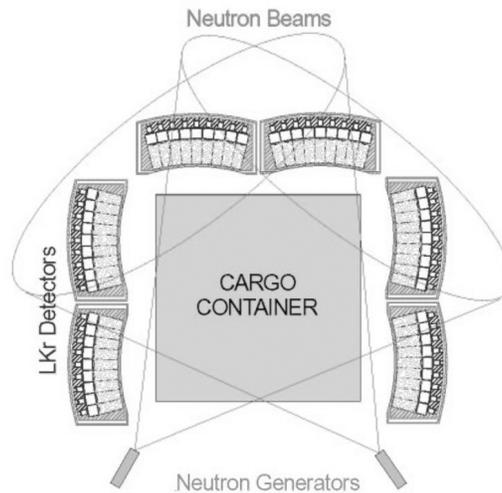
**Figure 1. Proposed neutron interrogation system [18].**
