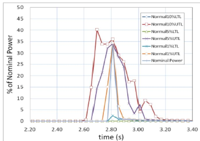
**Figure 6: Tolerance Intervals (95%,95%) for Normal Uncertainty in Cross-sections (*LTL*: Low Tolerance Limit, *UTL*: Upper Tolerance Limit).**
