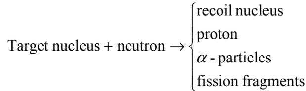
**Figure 1-1. Common reactions used for slow neutrons detection.**
