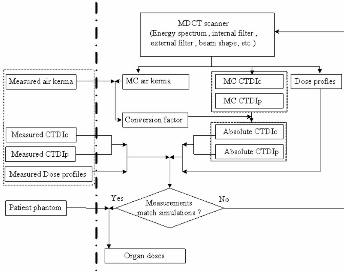
**Figure 1. Flowchart for development, validation and application of the MDCT models.**
