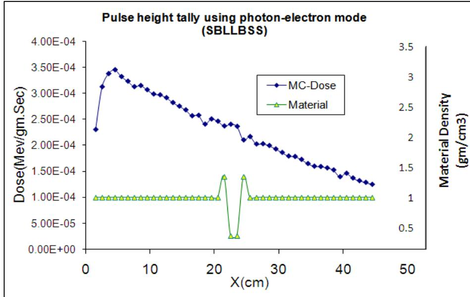
**Figure 4. Monte Carlo derived total absorbed dose rate distributions along the x-axis computed using \*F8 MCNP5 tally for the ‘SBLBSS’ slab phantom. MCNP uncertainty ( $2\sigma$ ) average (7.0%), 1000 Minute run, 16 processors.**
