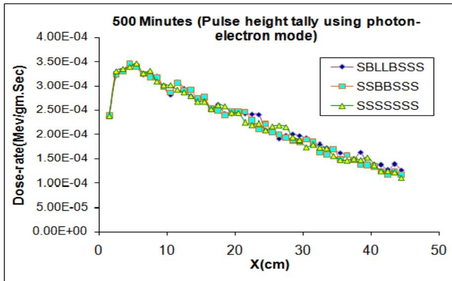
**Figure 3. Monte Carlo derived total absorbed dose rate distributions along the x-axis computed using \*F8 MCNP5 tally for three different phantoms. MCNP uncertainty ( $2\sigma$ ) average (10.0%), 500 Minute run, 16 processors.**
