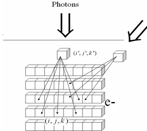
**Figure 1. Schematic of photons in a ‘dose driving voxel’ (DDV) at location  $(i',j',k')$  creating charged particles and energy deposition in voxels distal from the DDV**
