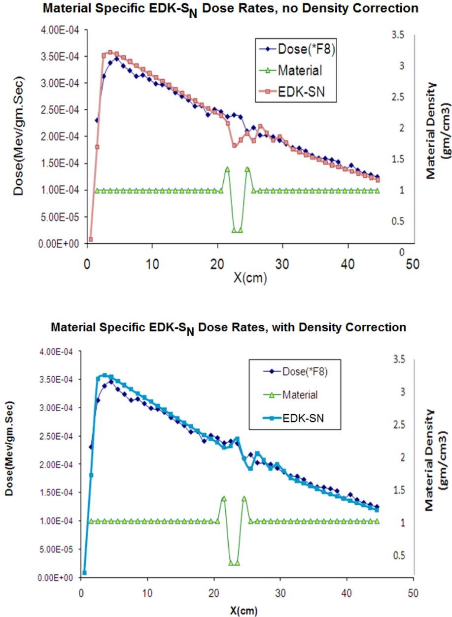
**Figure 6. (Top) EDK-S<sub>N</sub> Heterogeneous ‘S BLLBSS’ phantom total absorbed dose rate (without correction factor) along the x-axis compared to MCNP \*F8 tally dose rate. MCNP uncertainty ( $2\sigma$ ) average (8%) on-axis. Average absolute relative difference (4.1%); (Bottom) EDK-S<sub>N</sub> Heterogeneous ‘S BLLBSS’ phantom total absorbed dose rate with density correction applied, average absolute relative difference (<4.0%).**
