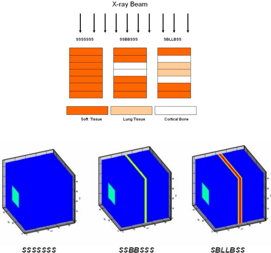
**Figure 2. (Top) Schematic of three phantoms for heterogeneous absorbed dose studies. Phantom SSSSSSS is a homogeneous soft-tissue (‘S’) phantom; phantoms SSBSSS and SBLLBSS include combinations of 1 cm sections of soft tissue (‘S’), bone (‘B’), and lung (‘L’) tissue-equivalent materials, respectively; (Bottom) 3-D model of the heterogeneous phantoms, and the beam source plane is shown on the left edge [14].**
