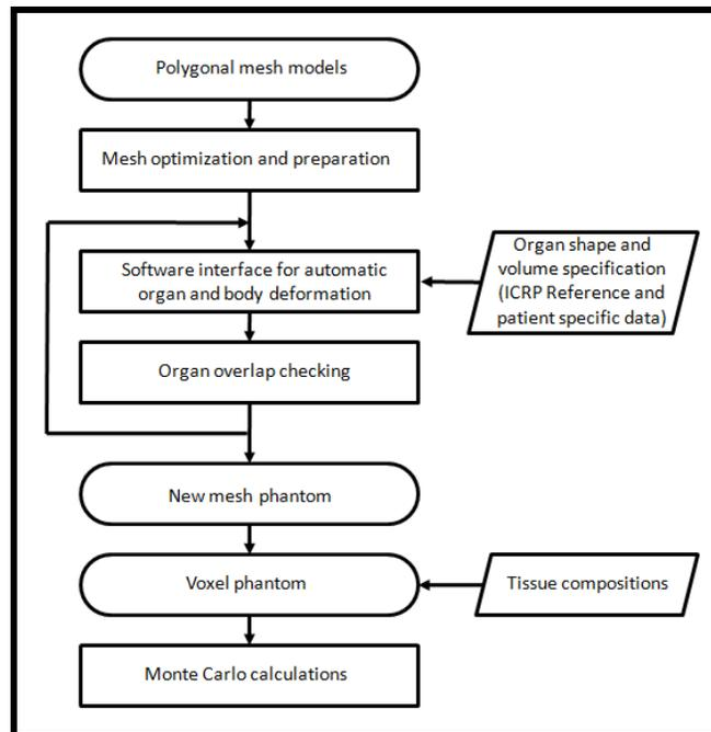
**Figure 1 Flowchart of the mesh-based modeling process used to develop adjustable phantoms.**
