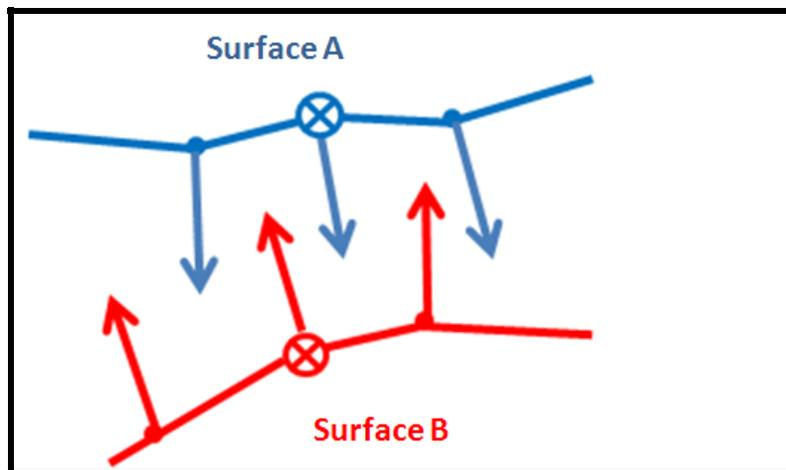
Figure 2 Illustration of the collision detection algorithm for Surfaces A and B represent two organ surfaces. A collision point between two surfaces occurs when the distance between a vertex (labeled as  $\otimes$ ) to the other surface along the normal direction is less than a pre-determined value. The detection continues until all the vertices on both surfaces have been examined this way.
