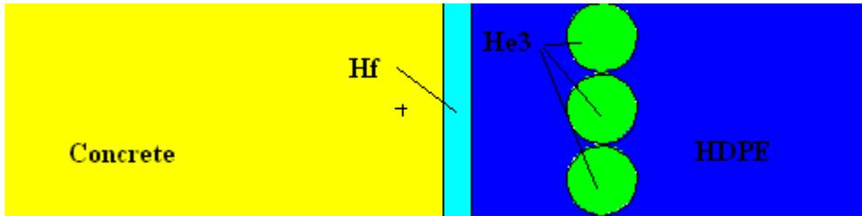
**Figure 6. Block II: 16 cm Concrete, 1 cm Hf filter materials, 12 cm HDPE.**
