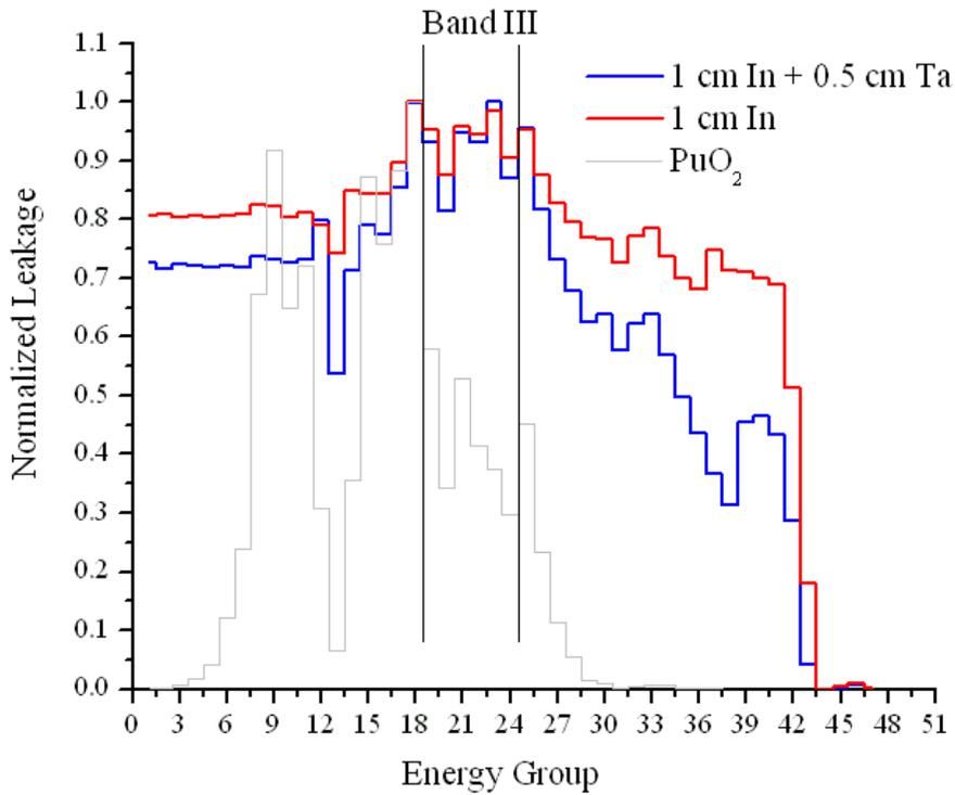
**Figure 3. Targeting Energy Band III by using 1 cm In and 0.5 cm Ta filter materials.**
