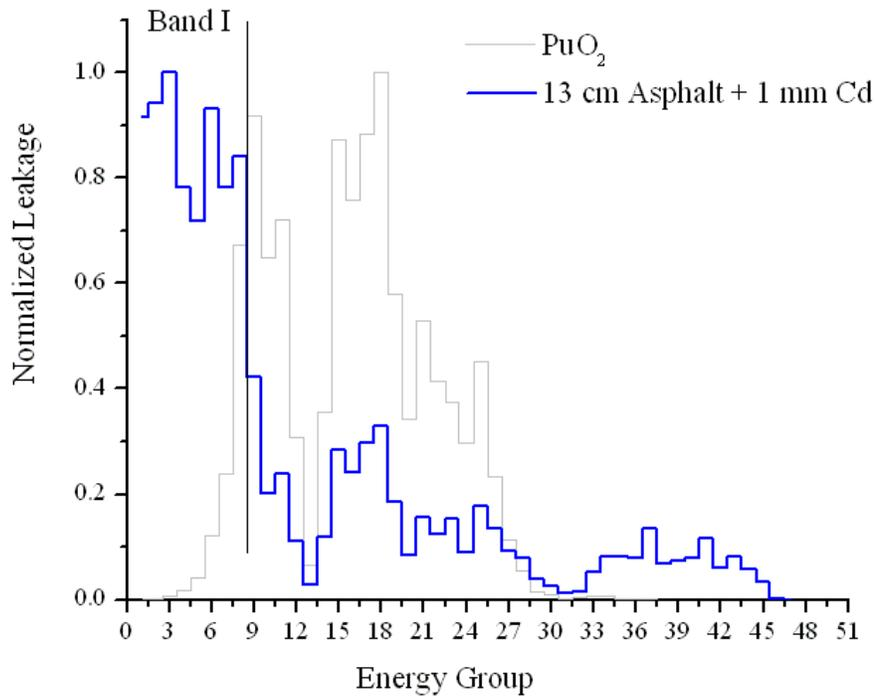
**Figure 7. Targeting Energy Band I by using 13 cm Asphalt and 1 mm Cd filter materials.**
