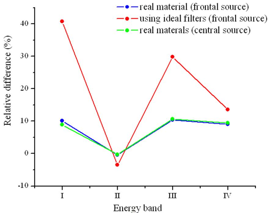
**Figure 9. Relative difference between Pu-metal and PuO<sub>2</sub> generated reaction rates using ideal filtering (red line) and when employing real materials (blue line) - frontal source, and real materials (green line) - central source.**
