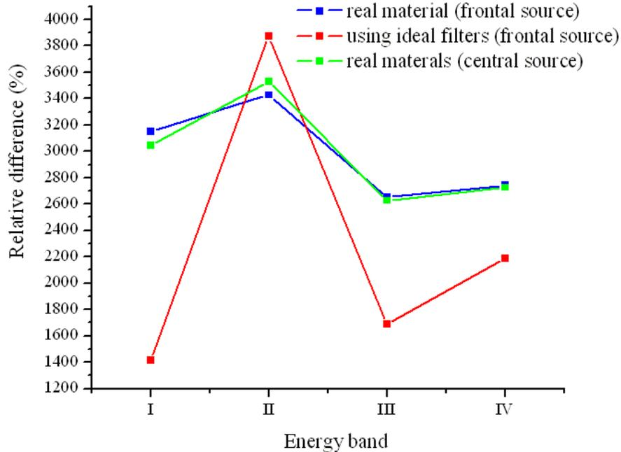
**Figure 10. Relative difference between U-metal and UO<sub>2</sub> generated reaction rates using ideal filtering (red line) when employing real materials (blue line) - frontal source, and real materials (green line) - central source.**
