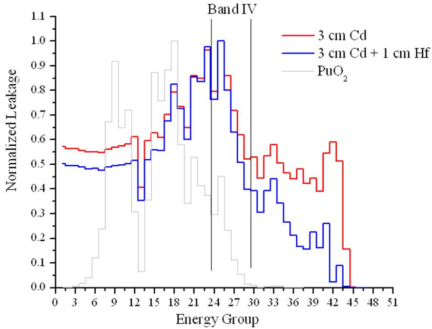
**Figure 1. Targeting Energy Band IV by using 3 cm Cd and 1 cm Hf filter materials.**
