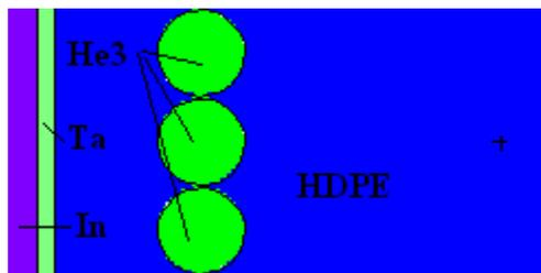
**Figure 4. Block III: 1 cm In and 0.5 cm Ta filter materials, 12 cm HDPE.**
