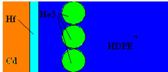
**Figure 2. Block IV: 3 cm Cd, 1 cm Hf filter materials, 12 cm HDPE.**
