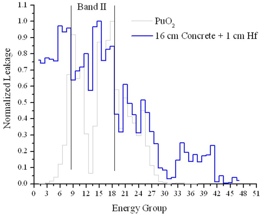
**Figure 5. Targeting Energy Band II by using 16 cm Concrete and 1 cm Hf filter materials.**
