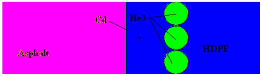
**Figure 8. Block I: 13 cm Asphalt, 1 mm Cd filter materials, 12 cm HDPE moderator.**
