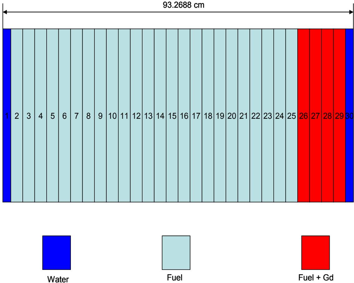
**Figure 3. 1-D BWR core configuration**
