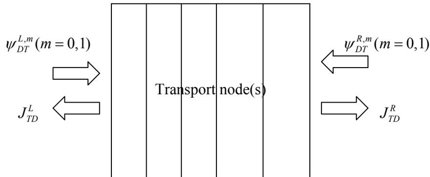
Figure 1. Coupling diffusion nodes to transport nodes
