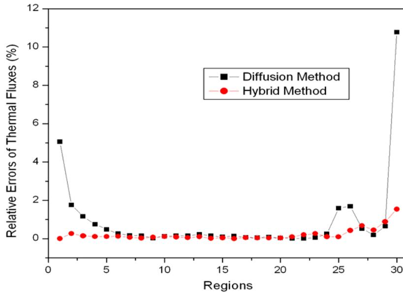
Figure 5. Relative error of the node-averaged thermal flux for each region
