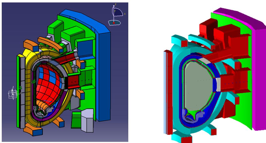
Figure 1 : ITER, 40° sector, left CATIA CAD model, right TRIPOLI model viewed in MCAM version 5, courtesy of ASIPP, FDS team
