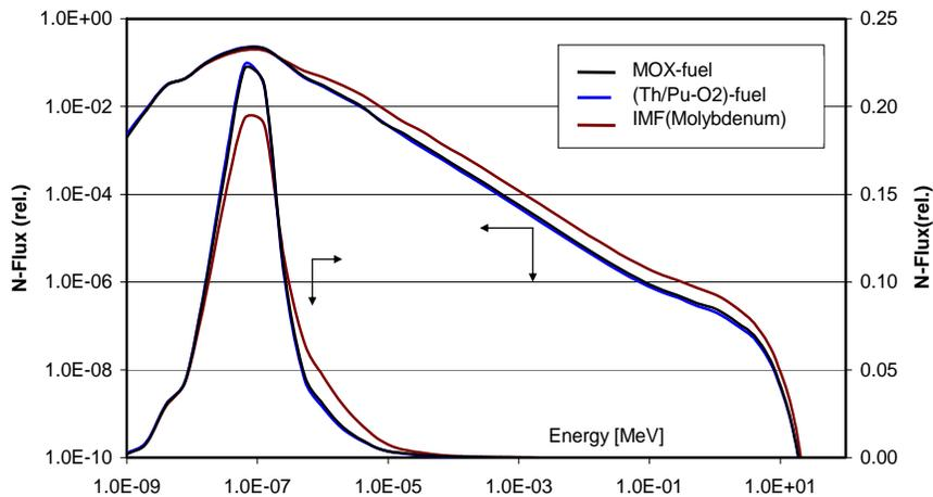
**Fig. 2: Comparison of the neutron spectrum in the fuel pin for different fuel types**
