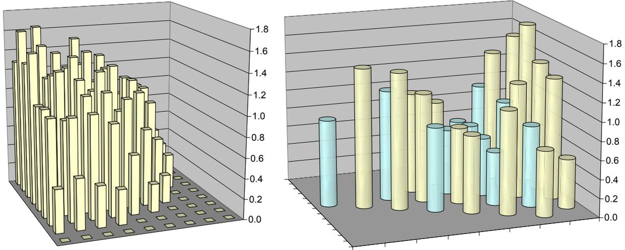
**Figure 3. Power distributions for one quarter of the uncontrolled state of the PWR core (left) and one sixth of the controlled state of the VVER core (right), calculated with JEFF-3.1 data. The distributions are normalized to the number of fuel assemblies. The core centre is on the left. Values for the controlled VVER fuel assemblies are marked in blue.**
