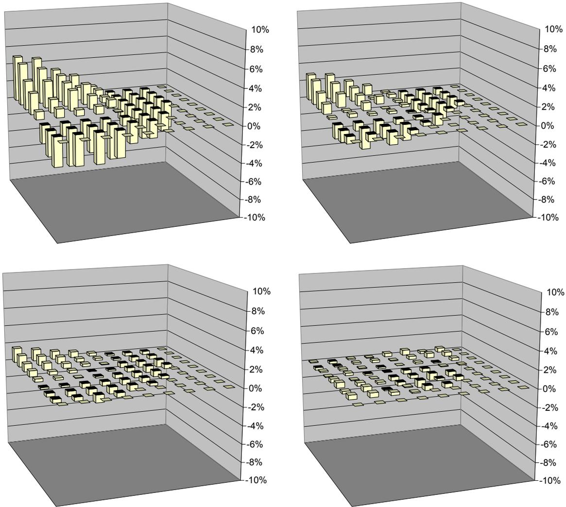
**Figure 5. Relative difference of the radial assembly power distributions for the uncontrolled state of the PWR UO<sub>2</sub>/MOX Core Benchmark, obtained with JEF-2.2 (top left), JENDL-3.2 (top right), ENDF/B-VII.0 (bottom left), and JENDL-3.3/AC-2008 (bottom right) as compared to results from JEFF-3.1 data.**
