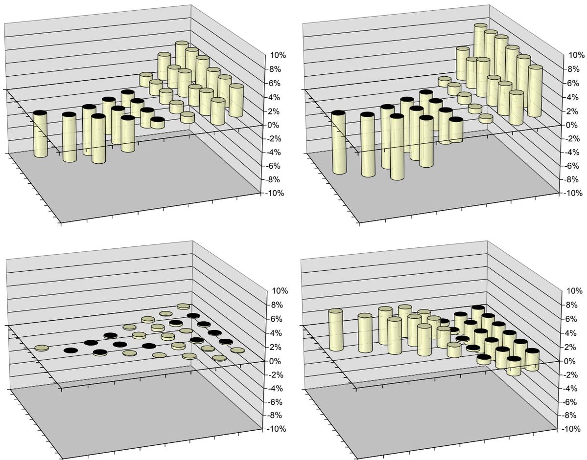
**Figure 6. Relative difference of the radial assembly power distributions for the uncontrolled state of the VVER-1000 MOX Core Benchmark, obtained with JEF-2.2 (top left), JENDL-3.2 (top right), ENDF/B-VII.0 (bottom left), and JENDL-3.3/AC-2008 (bottom right) as compared to results from JEFF-3.1 data.**
