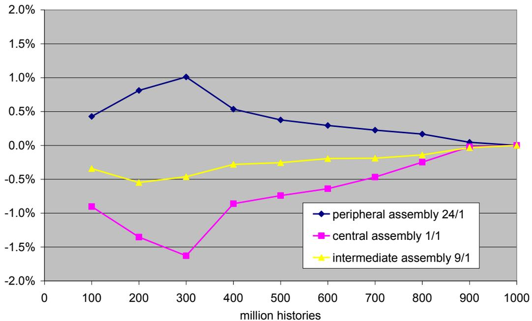
**Figure 4. Relative difference of the power of three VVER-1000 fuel assemblies from the final value after 1,000 million histories, as a function of neutron histories, obtained with JEFF-3.1 data.**
