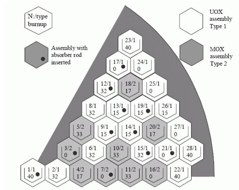
Figure 2. Core layout of the VVER-1000 MOX Core Computational Benchmark.
