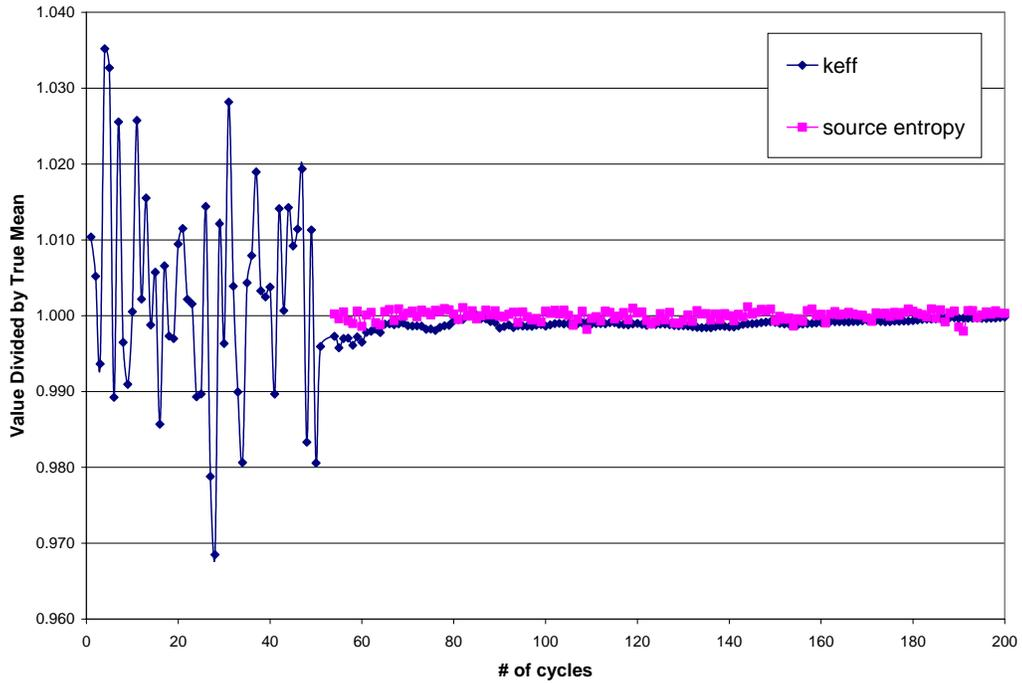
**Figure 7. Kozloduy-6 VVER Pin Cell Results with New Cross Sections**
