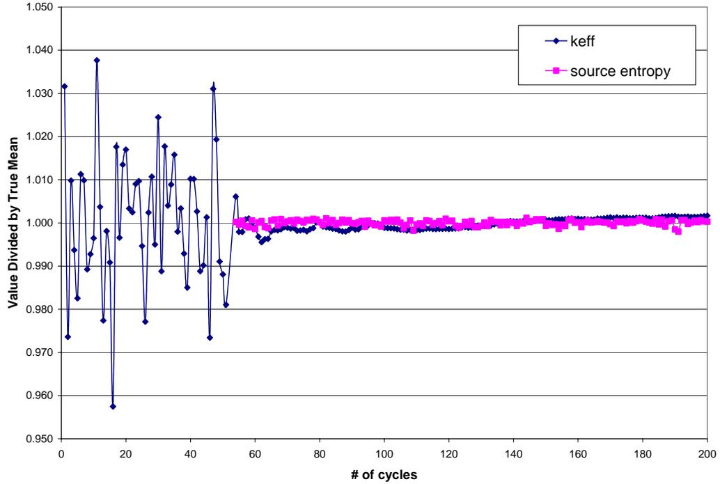
**Figure 6. PB-2 BWR 2D Pin Cell Results with New Cross Sections**
