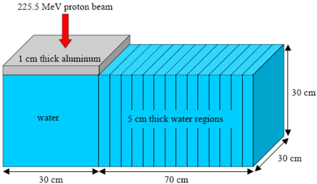
**Figure 4: Geometry for secondary neutron energy deposition calculations.**
