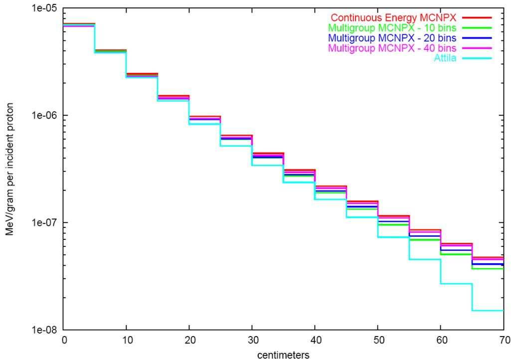
**Figure 5: Average neutron energy depositions in slab.**
