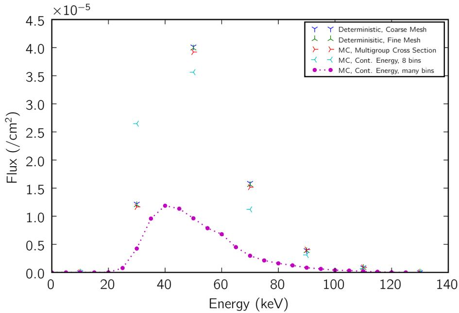
Figure 4: The computed flux at the center detector of the CTDI FDA phantom as computed with the constant-weighted multigroup cross section set.
