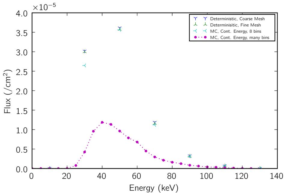
Figure 5: The flux at the center detector location of the CTDI FDA phantom as computed with the cross section set weighted by the flux spectrum computed by MCNP in the center of the phantom.
