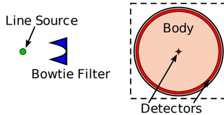
Figure 7: A cross section of the MCNP model with collimation and bowtie filter.
