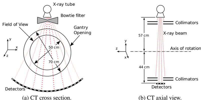
Figure 6: The essential structure of the CT machine. The dimensions are typical of most CT machines [19].
