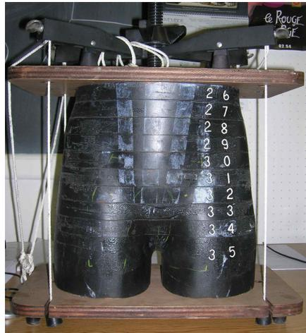
Figure 1: The Rando phantom anterior in its holding brace. The slice numbers are colored for better visibility.
