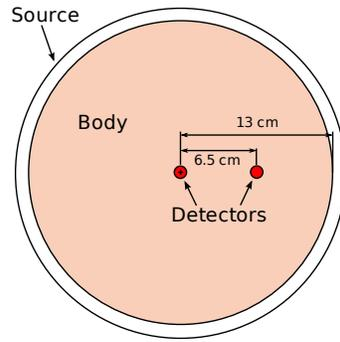
Figure 2: The simplified body cylinder MCNP model.
