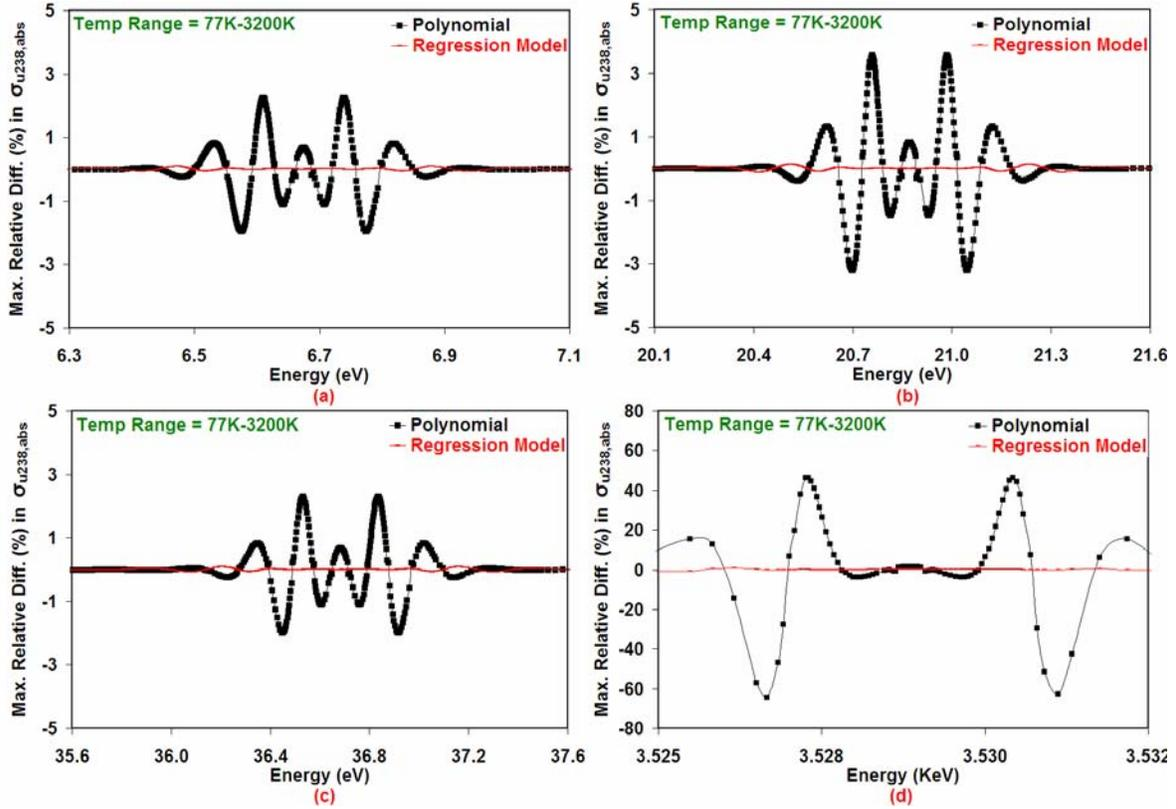
Figure 2. Maximum relative difference (%) for  $\sigma_a^{U238}$  at selected resonance energy grid points
