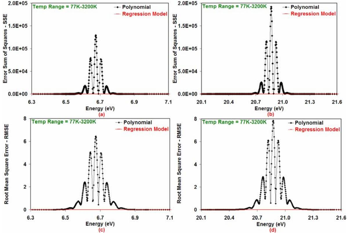
Figure 4. SSE and RMSE around selected important resonances of  $\sigma_a^{U238}$
