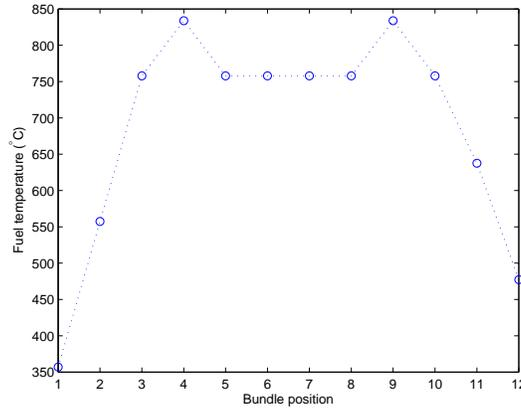
**Figure 5. Fuel Temperature vs. Bundle Position for *early* ACR-700**
