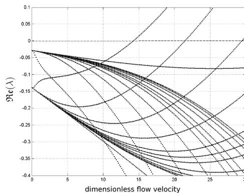
**Figure 6. Stability-parameter variation  $\Re\epsilon(\lambda)$  vs. dimensionless flow velocity**
