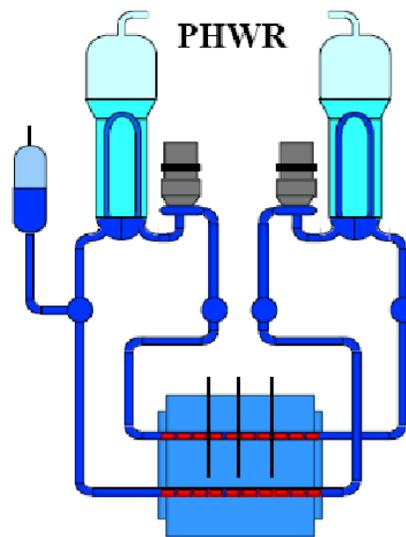
**Figure 1. A Coolant Loop in a CANDU Reactor [6].**
