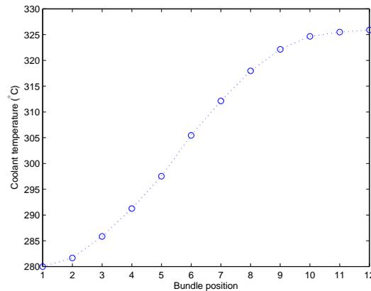
**Figure 4. Coolant Temperature *vs.* Bundle Position for *early* ACR-700**
