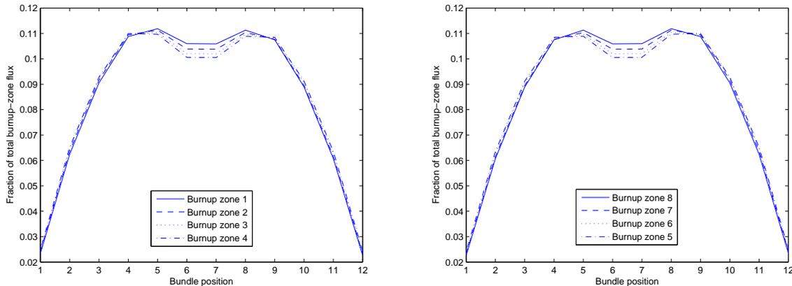
**Figure 7. Axial Flux for ACR-700 Refuelled in *Four-Bundle Shifts***
