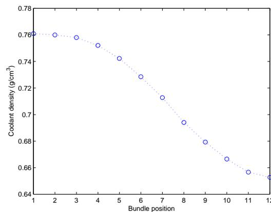
**Figure 3. Coolant Density vs. Bundle Position for *early* ACR-700**
