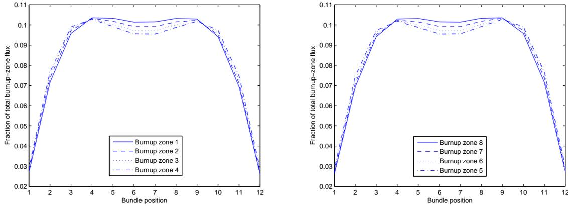
**Figure 8. Axial Flux for ACR-700 Refuelled in Two-Bundle Shifts**
