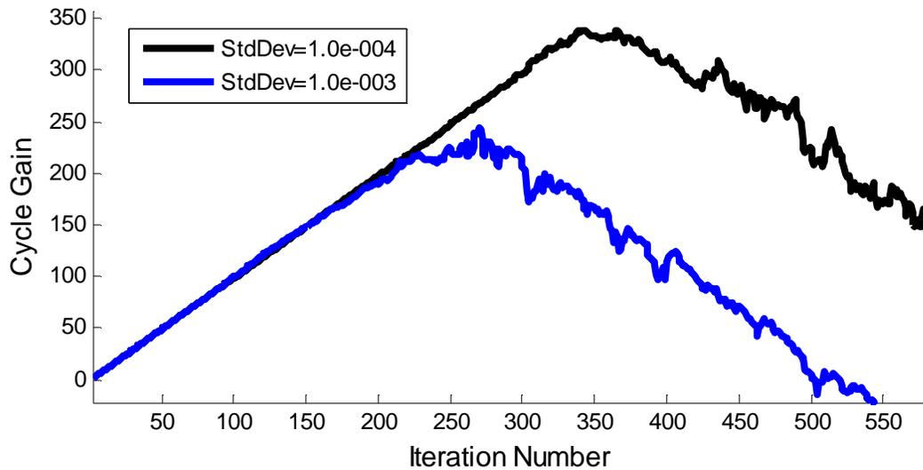
**Figure 2. Plot of modal gain for the first mode versus iteration for a system with dominance ratio 0.99 and  $\gamma_n = 1.0$  using  $\alpha = 0.98$  with two noise levels.**
