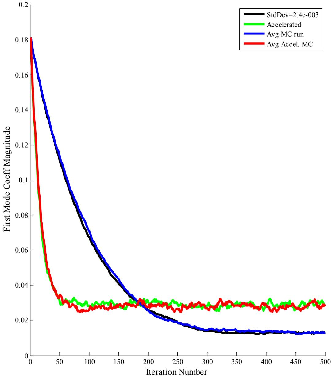
**Figure 4. Plot of the magnitude of the first mode eigenfunction decomposition coefficient versus iteration for a system with dominance ratio 0.99 and  $\gamma_1 = 0.18$  using  $\alpha = 4.0$  for acceleration. The MC lines indicate that the results are from a 1-D Monte Carlo simulation and the other two lines are expected from theory.**
