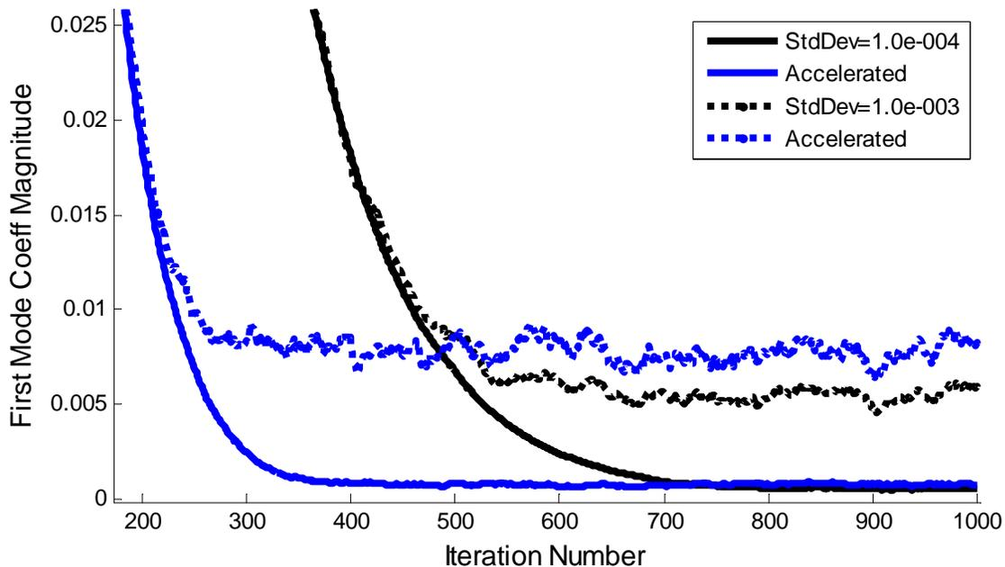
**Figure 1. Plot of first mode decomposition coefficient versus iteration for a system with dominance ratio 0.99 and  $\gamma_n = 1.0$  using  $\alpha = 0.98$  with two noise levels.**
