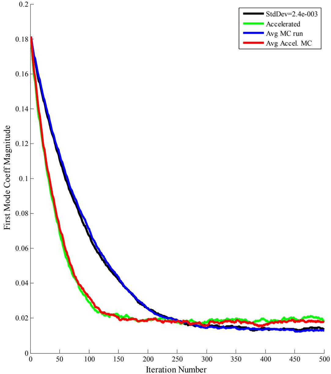
**Figure 3. Plot of the magnitude of the first mode eigenfunction decomposition coefficient versus iteration for a system with dominance ratio 0.99 and  $\gamma_I = 0.18$  using a conservative extrapolation parameter,  $\alpha = 0.98$ , for acceleration. The MC lines indicate that the results are from a 1-D Monte Carlo simulation and the other two lines are expected from theory.**
