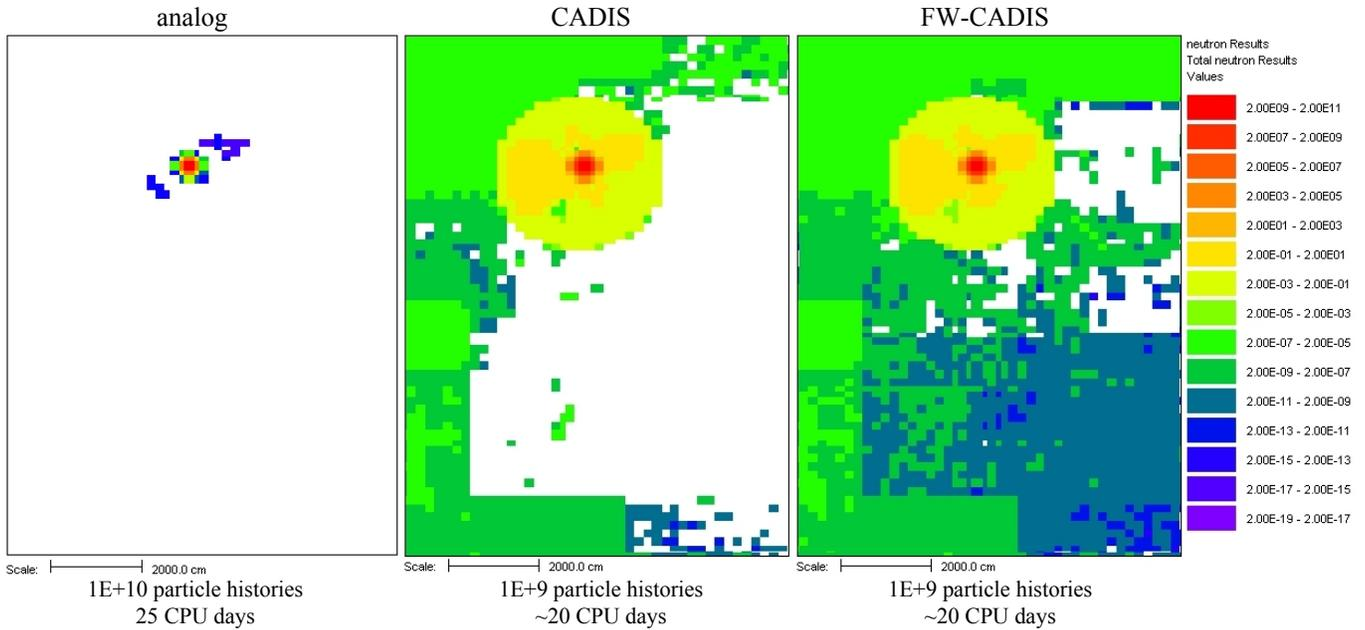
**Figure 2. Dose rates (mrem/h) computed using analog (left), CADIS with the adjoint source on the outer boundaries of the model (center), and FW-CADIS (right).**
