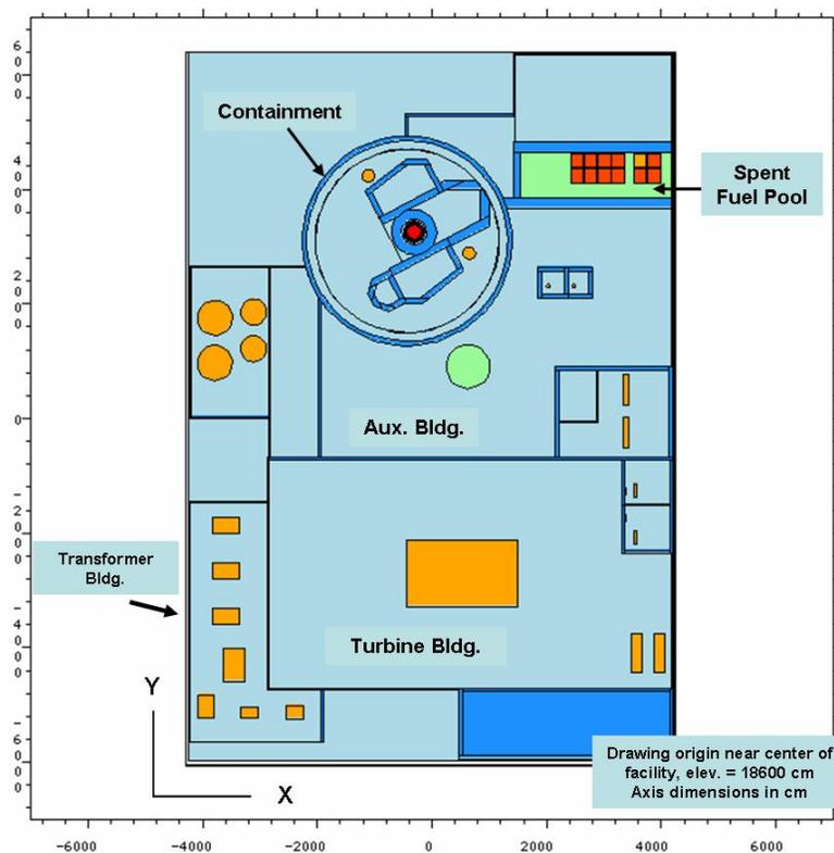
**Figure 1. Plan X-Y view of PWR facility MCNP model. The containment, auxiliary, and turbine buildings and major components are shown.**
