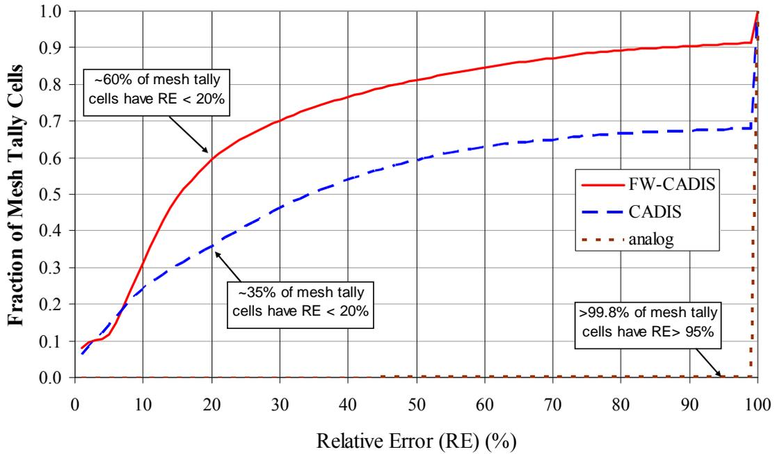
Figure 4. Relative error histograms for the different methods.
