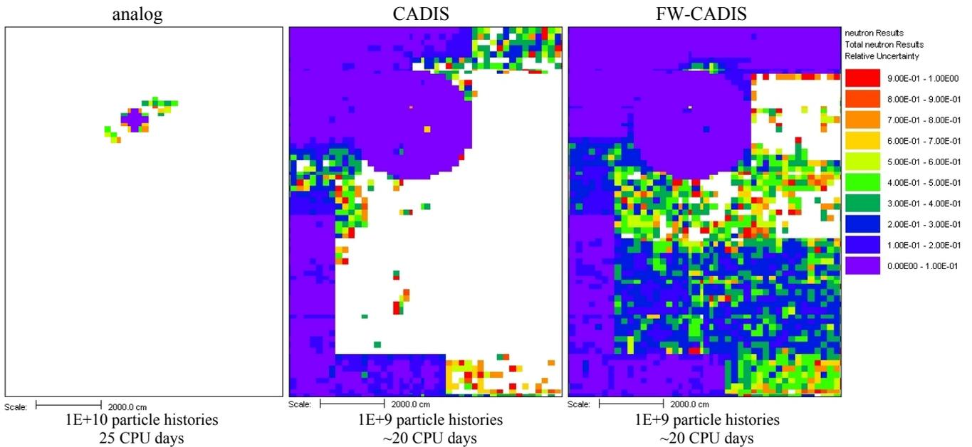
**Figure 3. Relative errors computed using analog (left), CADIS with the adjoint source on the outer boundaries of the model (center), and FW-CADIS (right).**
