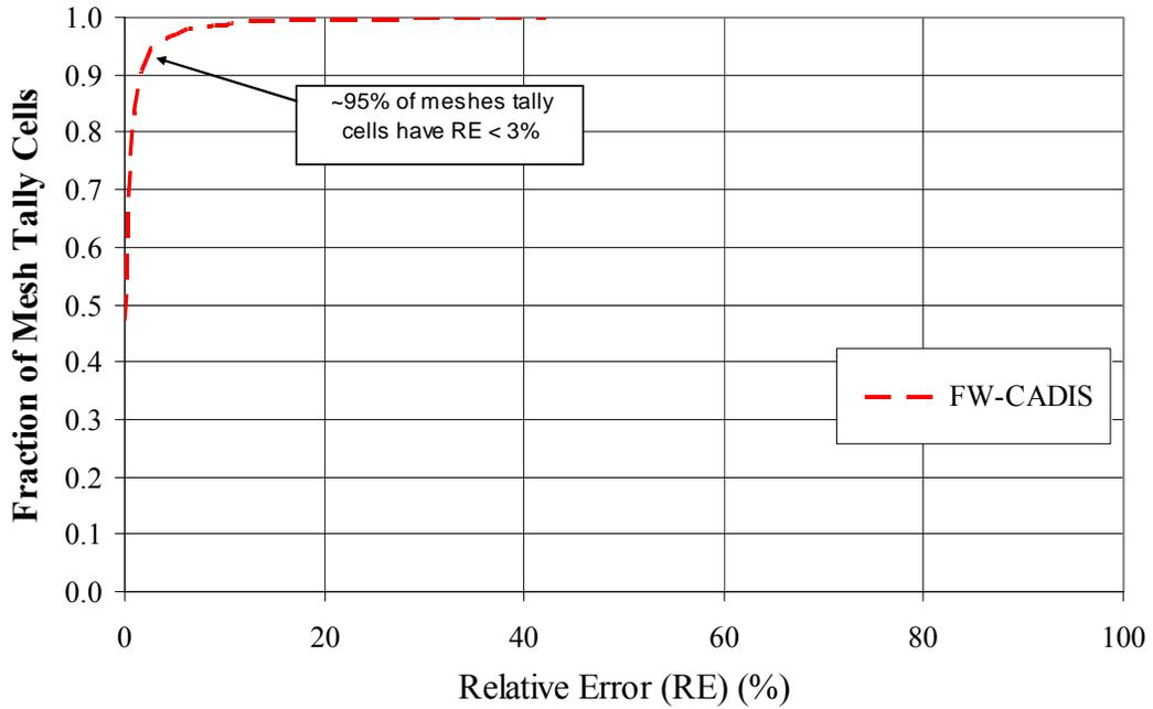
Figure 5. Relative error histogram for tally cells with dose rates  $\geq 1$  mrem/h.
