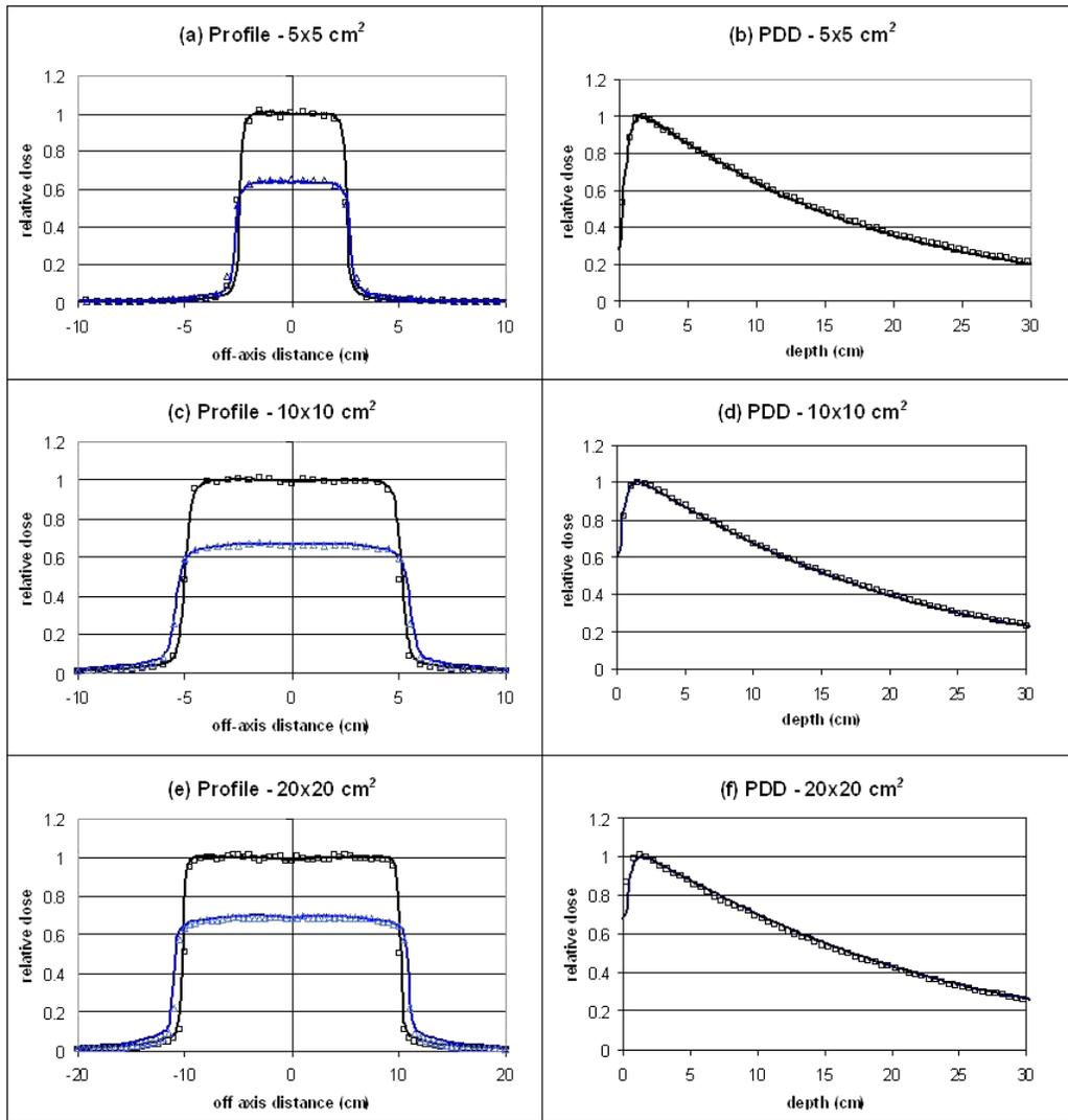
**Figure 3. Calculated and measured dose curves. The profiles are at 1.5 cm deep (black) and 10 cm deep (blue). In all graphs, the solid lines represent the measurements while the squares and the triangles are calculated with the directional spectrum model. The error bars are not shown for clarity. All relative errors are below 10%.**
