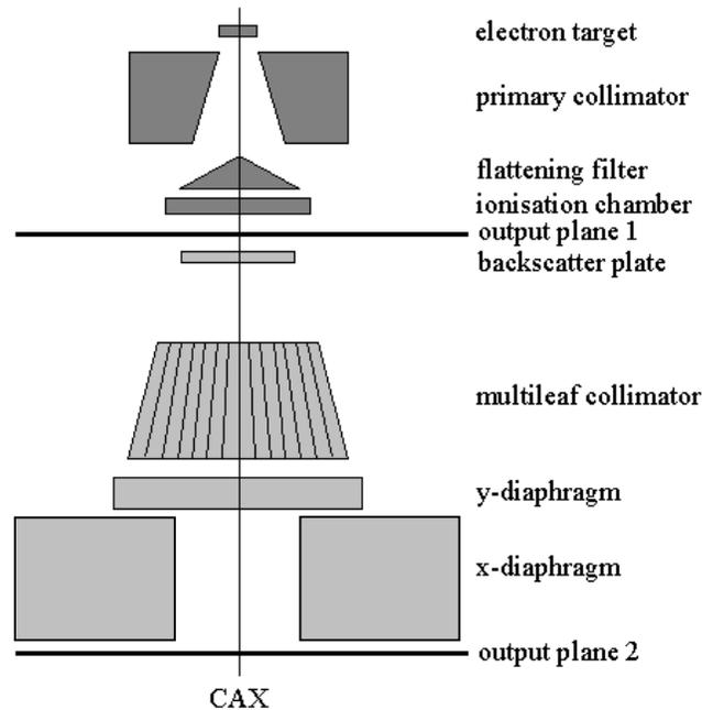
**Figure 1. Schematic diagram of an Elekta SLi linac. Output plane 1 is where our directional spectrum model applied. Output plane 2 is used for further simulations downstream.**
