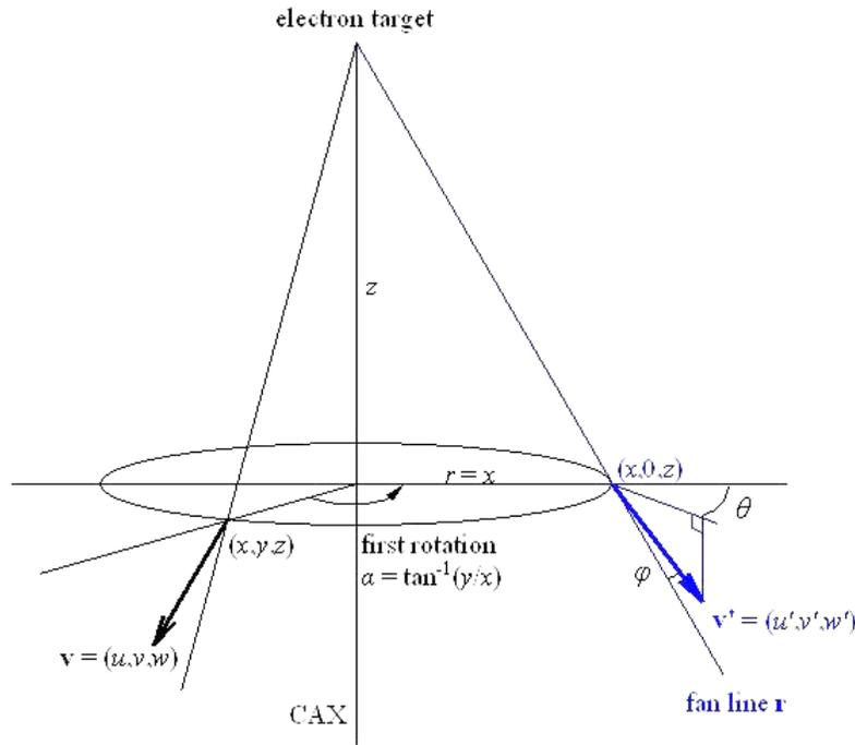
**Figure 2. The directional spectrum model. The particles are compressed onto the x-axis and the energy spectrum is associated with the radial position  $r$  and the normalized scattering angle  $\varphi$ . The azimuthal angle  $\theta$  has no importance in the model.**
