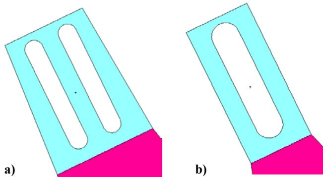
Figure 4. Outer parts of PO-3 rotors as used in the MCNP geometry model. a) Main reflector (I). b) Auxiliary reflector (II).
