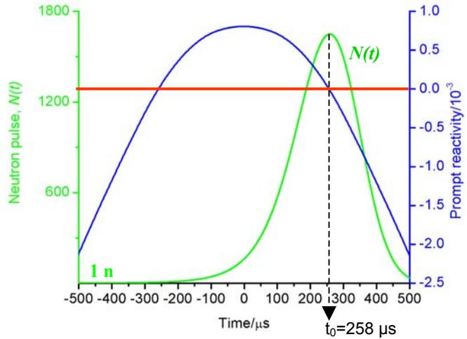
Figure 2. Courses of prompt reactivity and of fast neutron pulse (started with 1 neutron) in IBR-2 for the standard regime with the reflector system PO-2.
