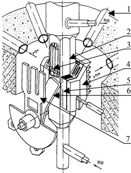
Figure 1. Schematic outline of the IBR-2 with reflector PO-2. 1 neutron channel, 2 reactor tank, 3 reactor core, 4 moderators, 5 stationary reflector with control elements, 6 main reflector, 7 auxiliary reflector.
