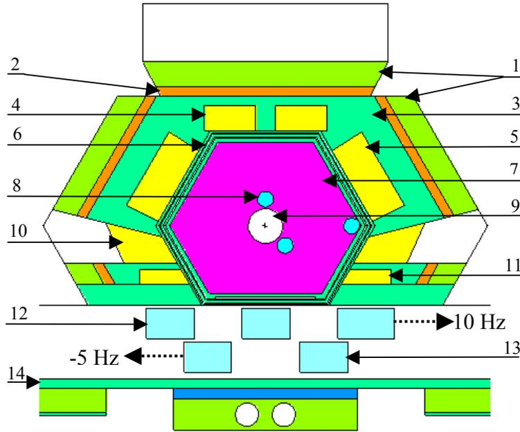
Figure 3. Horizontal cross-section of IBR-2 with the new reflector system PO-3 as used in the MCNP geometry model. 1 water moderators, 2 boron carbide, 3 stationary reflector, 4 slow shutoff element, 5 control element, 6 double wall core tank, 7 core, 8 dummy element, 9 central channel, 10 fast shutoff element, 11 operator control element, 12 main reflector (I), 13 auxiliary reflector (II), 14 case of the rotating reflector.
