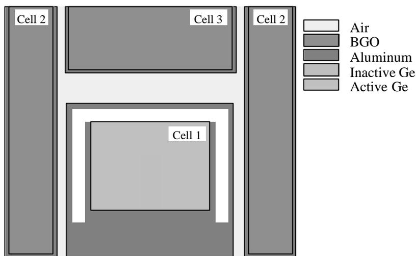
**Figure 1. Model of a hypothetical Compton suppression system on the basis of HPGe analyzing detector.**
