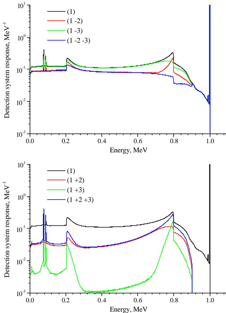
**Figure 2. Compton suppression spectrometer responses calculated for different guard detector and spectrum acquisition modes combinations (results of 10<sup>7</sup> trials).**
