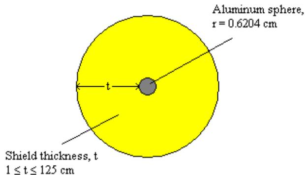
**Figure 3. Schematic of the spherical shielding geometry employed in these Monte Carlo calculations. A shield of varying thickness, t, was placed around an isotropic source at the center of an aluminum sphere.**
