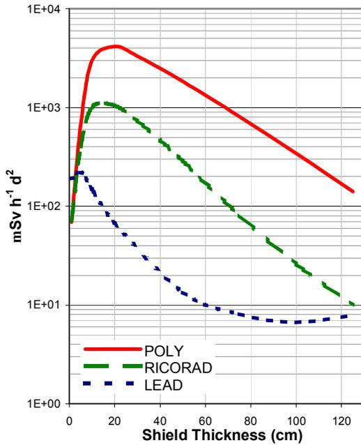
Figure 6. Equivalent dose to ICRU four-component tissue from secondary gamma rays (neutron capture photons) for the three shielding materials.
