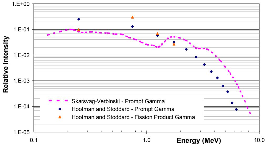
**Figure 2. Prompt and delayed photon emission spectrum from spontaneous fission of  $^{252}\text{Cf}$  and decay of fission daughter products, respectively. The prompt gamma ray spectrum measured by Skarsvåg and modified using data by Verbinski *et al.* was used in this study.**
