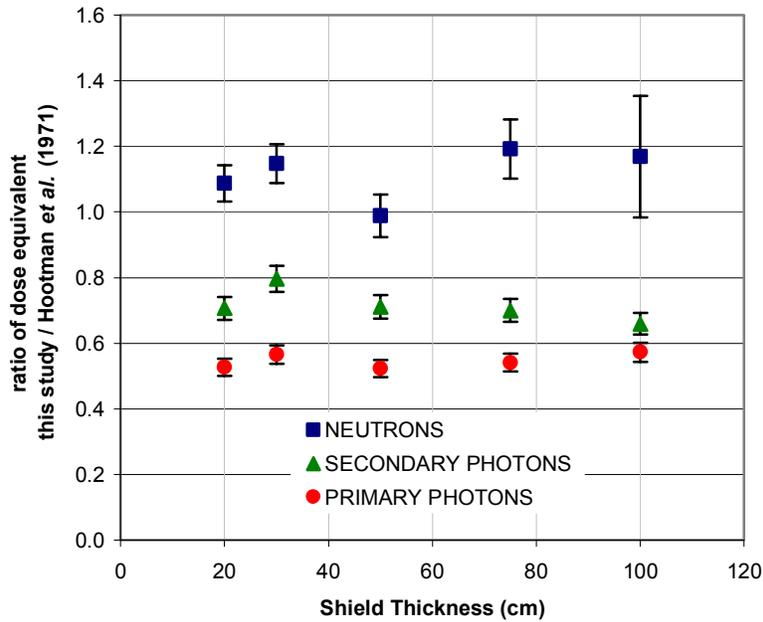
**Figure 8. Ratio of Monte Carlo shielding calculations for polyethylene from this study to Hootman and Stoddard (1971).**
