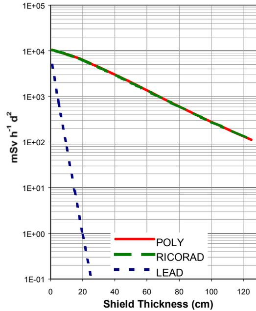
Figure 5. Equivalent dose to ICRU four-component tissue from primary gamma rays for the three shielding materials.
