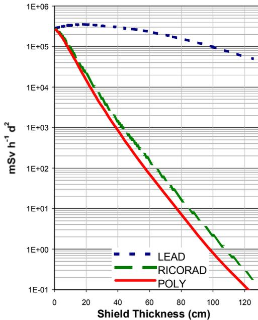
Figure 4. Equivalent dose to ICRU four-component tissue from <sup>252</sup>Cf neutrons for the three shielding materials.
