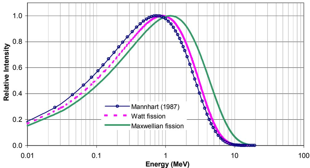
**Figure 1. Comparison of normalized Mannhart  $^{252}\text{Cf}$  neutron emission spectrum, Watt fission spectrum, and Maxwellian fission spectrum. In this study, the Mannhart neutron spectrum was utilized.**
