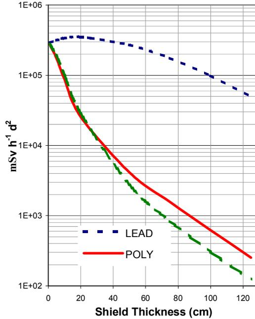
Figure 7. Total equivalent dose to ICRU four-component tissue after attenuation through Pb, polyethylene, and RICORAD™.
