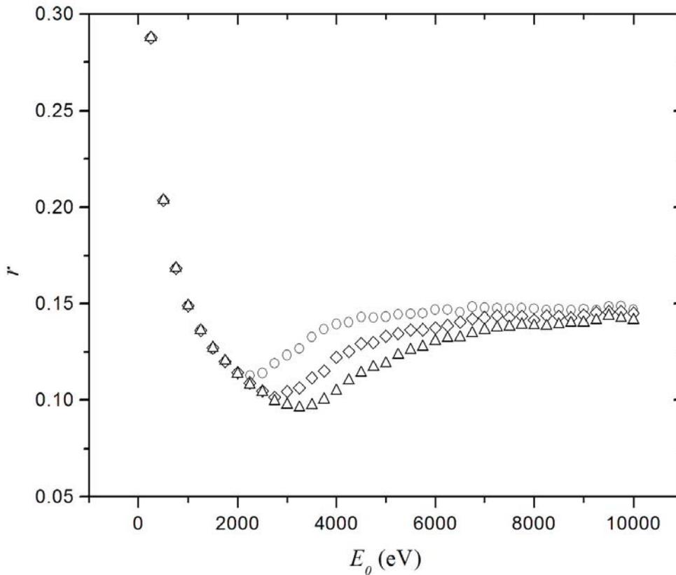
**Figure 2. Monte Carlo simulation of the electron backscattering coefficient  $r$  for C films deposited on Al substrates as a function of the beam primary energy  $E_0$ . C film thickness: 400 Å (circles), 600 Å (diamonds), and 800 Å (triangles).**
