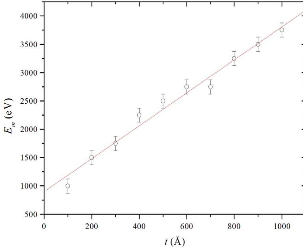
**Figure 4.** Energy  $E_m$  of the relative minimum of the backscattering coefficient as a function of the film thickness  $t$  for C films deposited on Al substrates. Circles with the error bars represent the calculated data. The line is the best linear fit:  $E_m = a t + b$  where  $a = 2.9 \pm 0.1$ ,  $b = 900 \pm 90$ .
