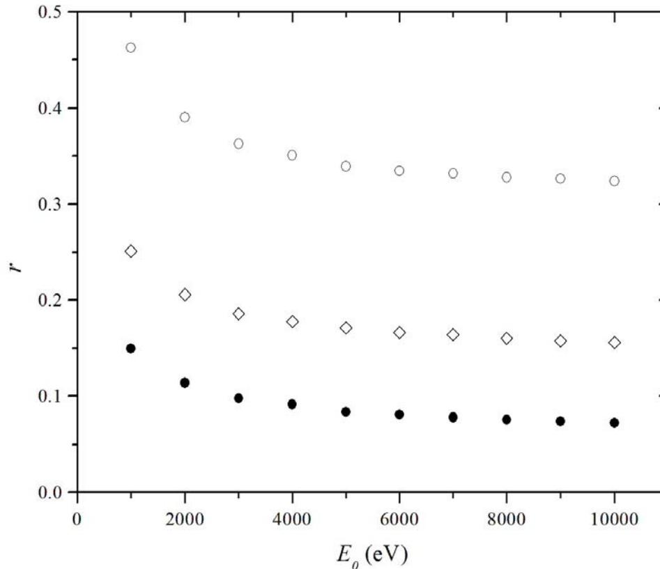
**Figure 1. Monte Carlo simulation of the backscattering coefficient  $r$  as a function of the primary energy  $E_0$  for electrons impinging on bulk targets of C (bullets), Al (diamonds), and Cu (circles).**
