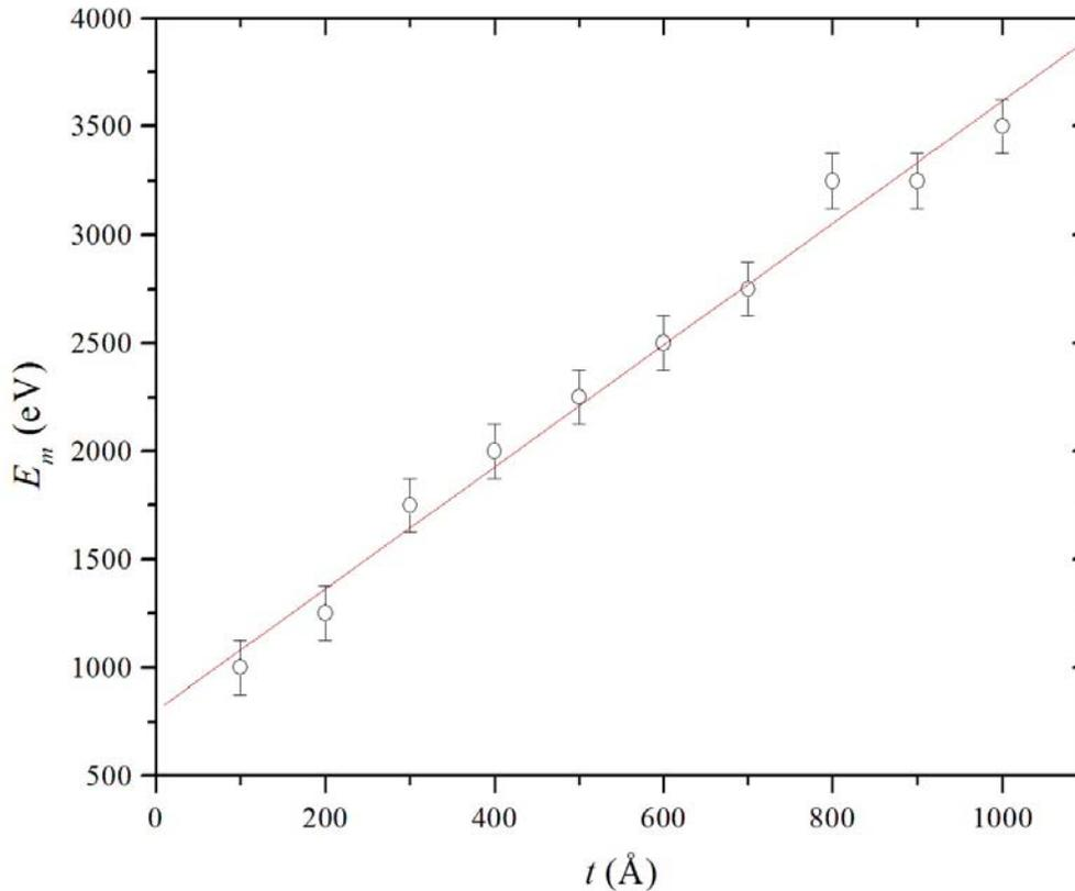
**Figure 5.** Energy  $E_m$  of the relative minimum of the backscattering coefficient as a function of the film thickness  $t$  for C films deposited on Cu substrates. Circles with the error bars represent the calculated data. The line is the best linear fit:  $E_m = a t + b$  where  $a = 2.8 \pm 0.1$ ,  $b = 800 \pm 75$ .
