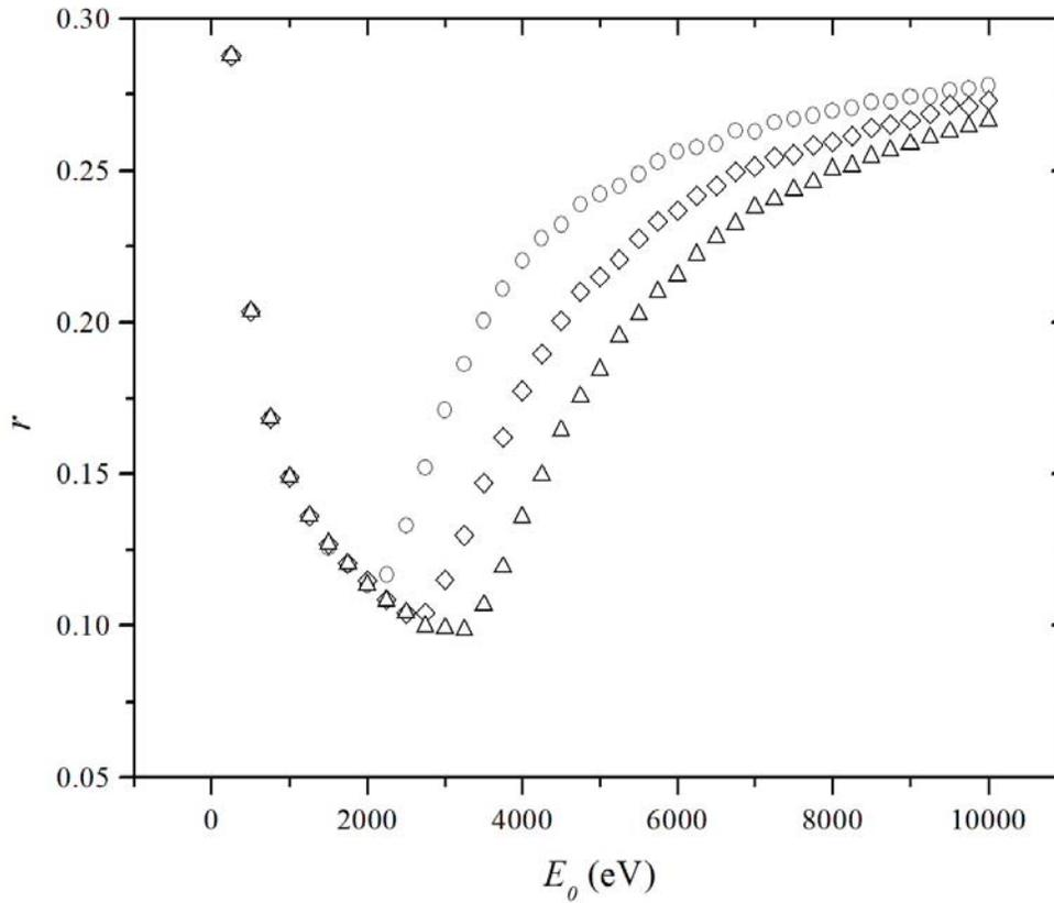
**Figure 3. Monte Carlo simulation of the electron backscattering coefficient  $r$  for C films deposited on Cu substrates as a function of the beam primary energy  $E_0$ . C film thickness: 400 Å (circles), 600 Å (diamonds), and 800 Å (triangles).**
