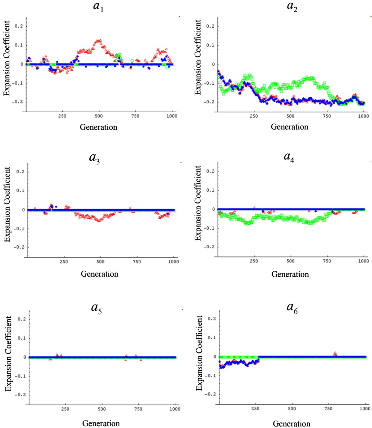
Figure 7. Filtered low order Legendre moments of the fission source by generation for thermal-spectrum critical assembly. Results are shown for the cost-to-benefit ratio filter threshold values of 0.95 (red), 0.6 (blue), and 0.3 (green). All results were generated in independent Monte Carlo criticality calculations using collision FET source sampling with 1000 generations and 100,000 histories per generation.
