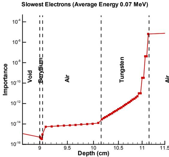
**Figure 9 Electron Importance in the Flattening Filter**
