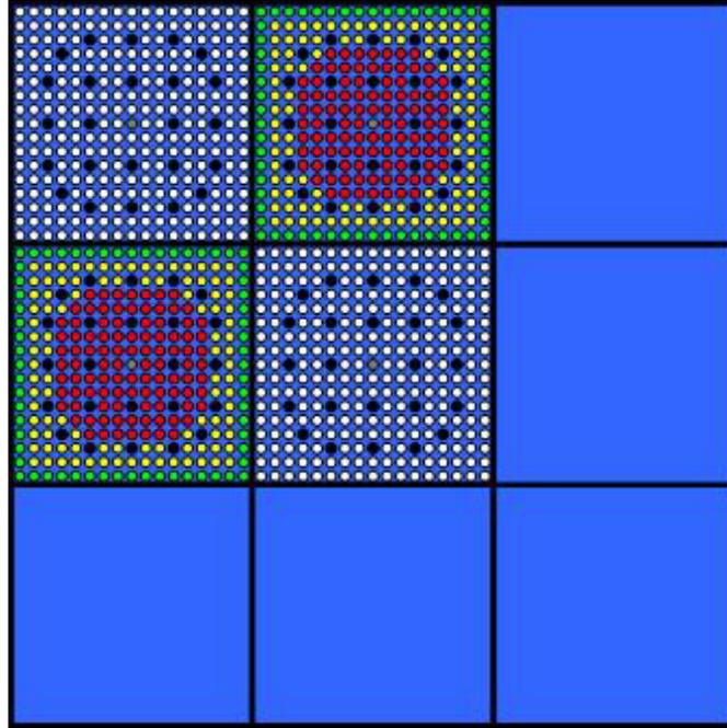
**Figure 3: Geometrical Configuration of the C5G7 2-D MOX Benchmark Problem**
