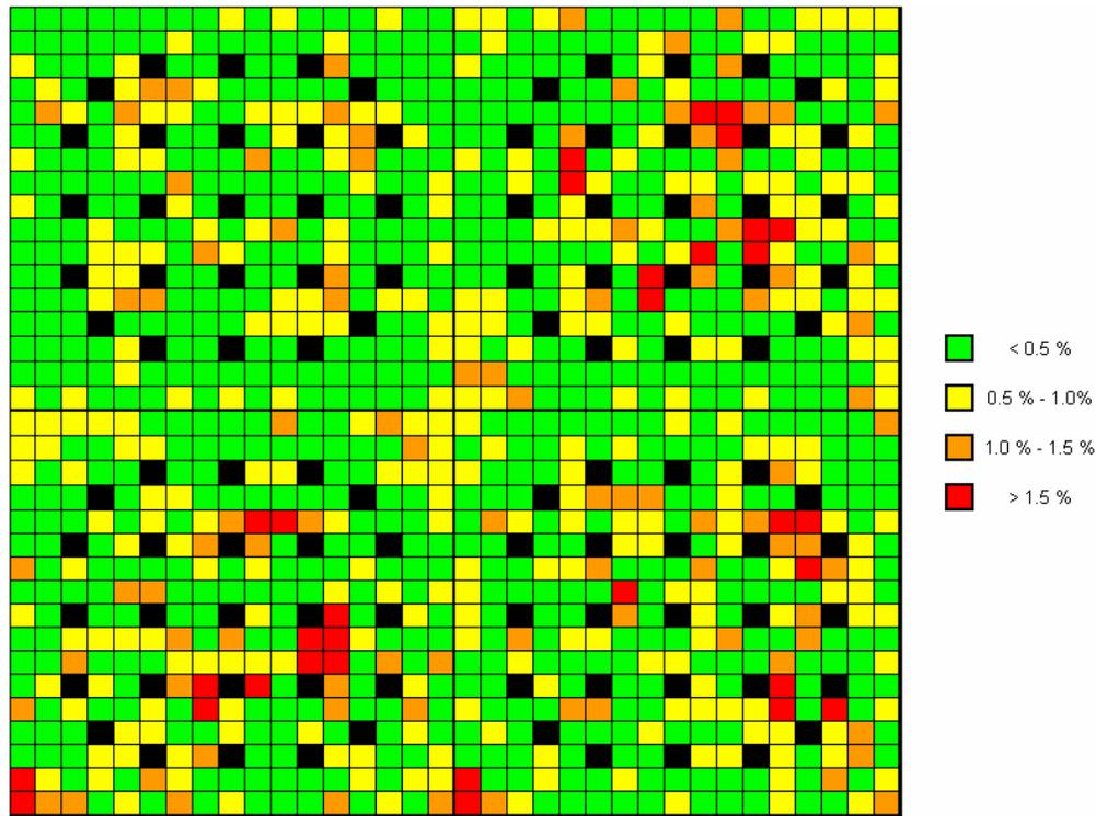
**Figure 4: Relative Error Distribution of the Pin Powers of the C5G7 2-D MOX Benchmark for the  $\{2,2,2\}$  case.**
