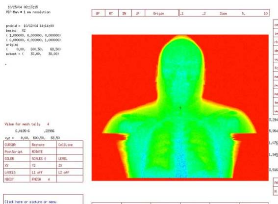
Figure 3. A transmission radiograph of 1mm<sup>3</sup> VIP-Man torso from 120 kVp x-ray source
